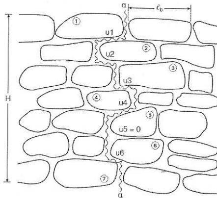
Fig. 5: Bonding may be quantified by summing up the overlapping lengths 'u<sub>i</sub>' along a quasi-vertical section  $\alpha\text{-}\alpha$
