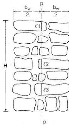
Fig. 8: The vertical axis p-p of the transversal cross-section intersects only relatively long blocks (lengths  $l_1, l_2, l_3$ )
