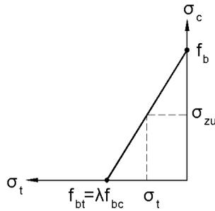
Fig. 2: Critical combination of compressive and tensile stresses acting on the block
