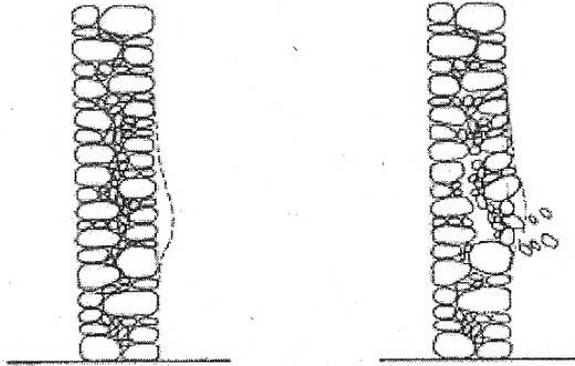
Fig. 7: Possible bulging on unbonded 'faces' of masonry (A. Giuffr )
