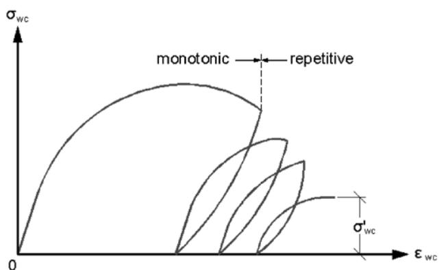
Fig. 11: Repetitive compression applied after the failure under monotonic loading
