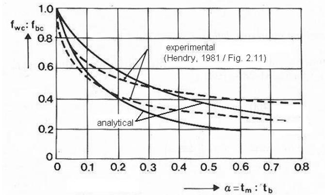
Fig. 3: Reduction of compressive strength of brick masonry, due to larger widths of mortar joints
