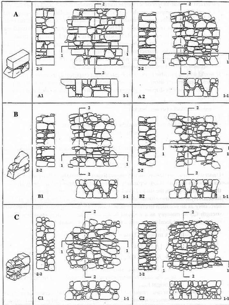
Fig. 9: Bonding models useful to 'calibrate' a given masonry wall and 'classify' it in a suitable 'quality class' A, B or C. (Italian Guidelines)
