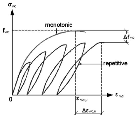
Fig. 10: Repetitive compression applied since the beginning of loading
