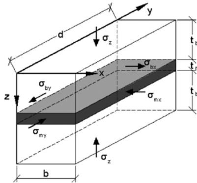
Fig. 1: Endogenous stresses in a masonry element under uniaxial external compression  $\sigma_z$
