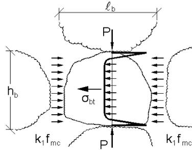
Fig. 4: In extremis, a rubble stone may be seated on its supporting stone on one point only
