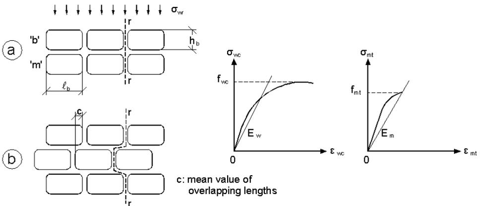
Fig. 6: Generation of a vertical crack r-r within mortar, due to the incompatibility of horizontal strains
