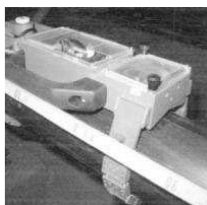
Figure 8: Free length internal inspection by using a special sensor (capacitive gauge inspection)
