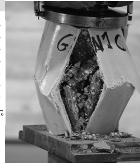
Collapse of hybrid short column
