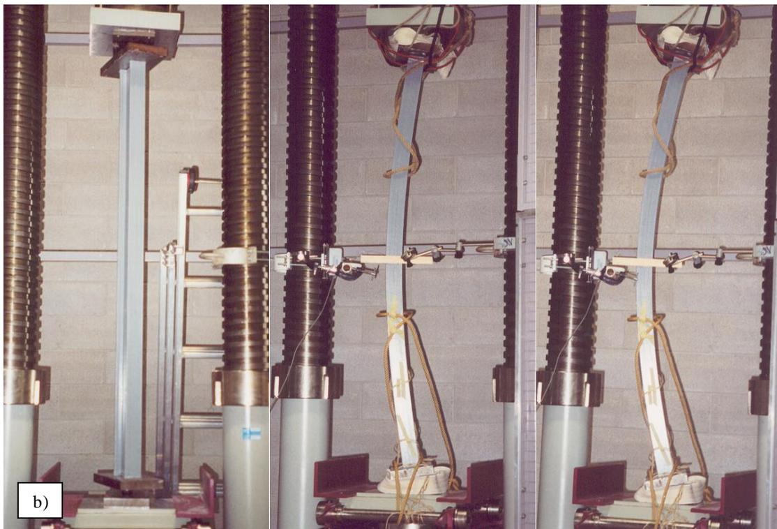
Figure 3. a) Load-axial displacement curve also with lateral displacement curves (coloured and on the left) at the half of the column; b) failure mode. FRP column, "I" shape;  $h = 1500 \text{ mm}$
