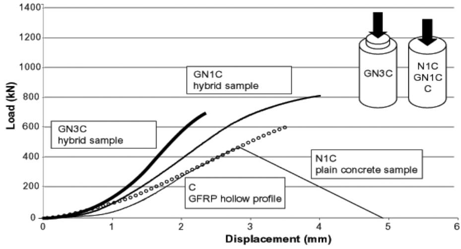
Figure 7. Load displacements curves for short circular samples with and without concrete
