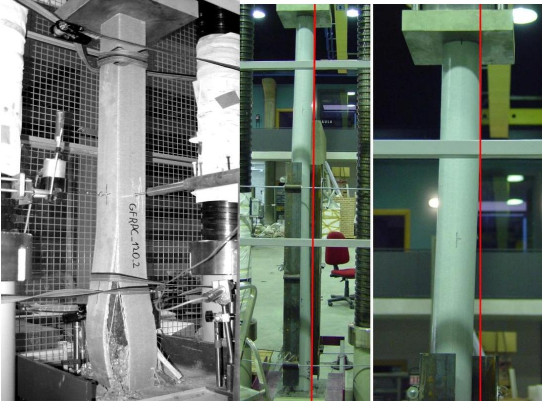
Figure 8. Collapse of FRP/Concrete columns with square and circular cross section; high values of  $\lambda$
