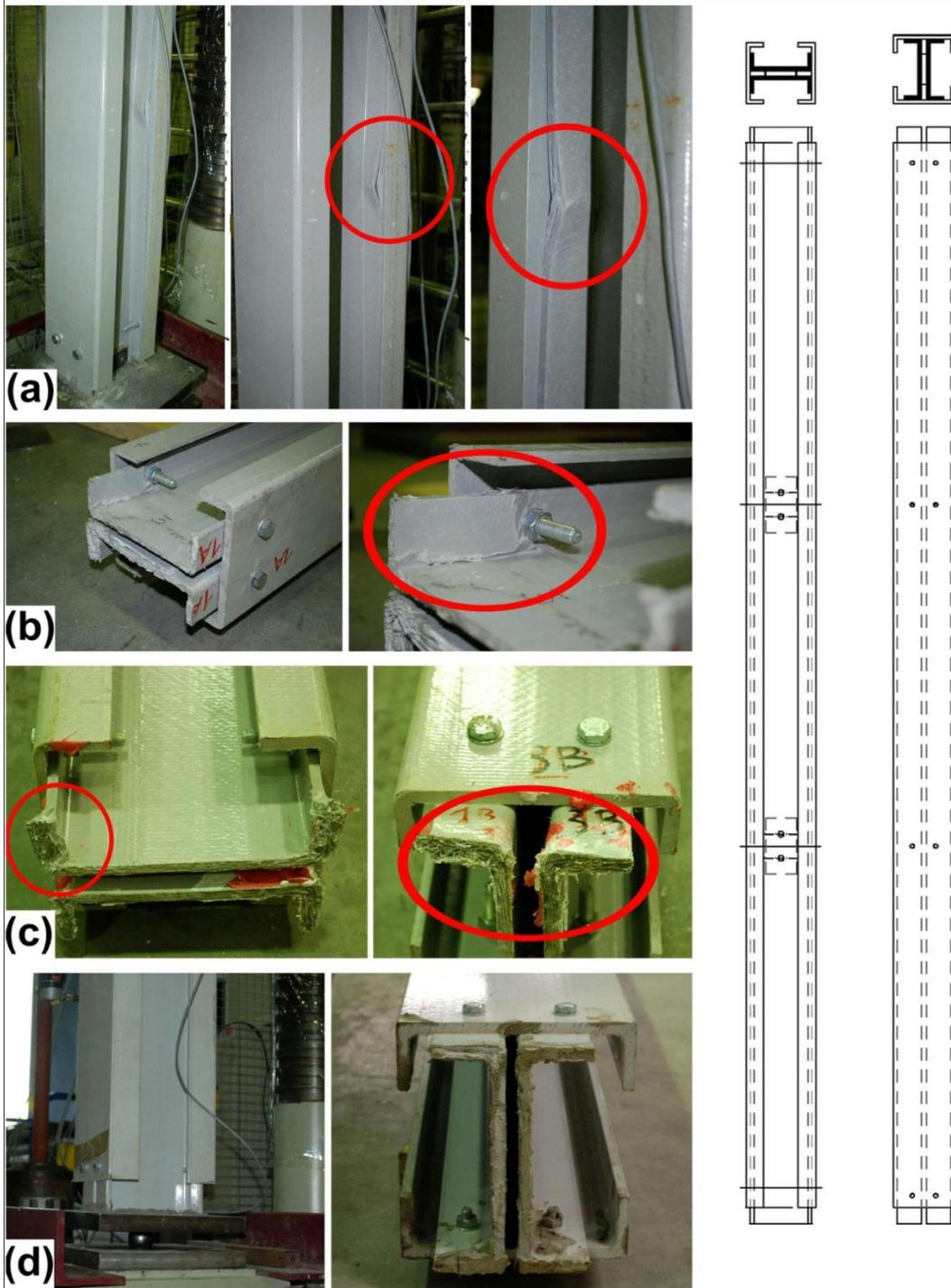
Figure 10. Loca/ global failure modes for built-up columns; load appli
