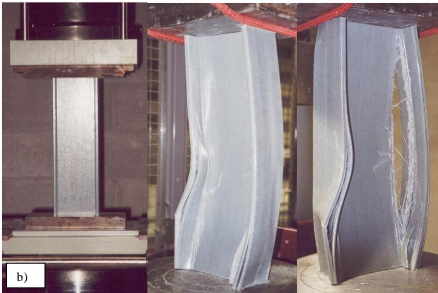
Figure 2. a) Load-axial displacement curve; b) failure mode. FRP column, "I" shape,  $h = 360 \text{ mm}$
