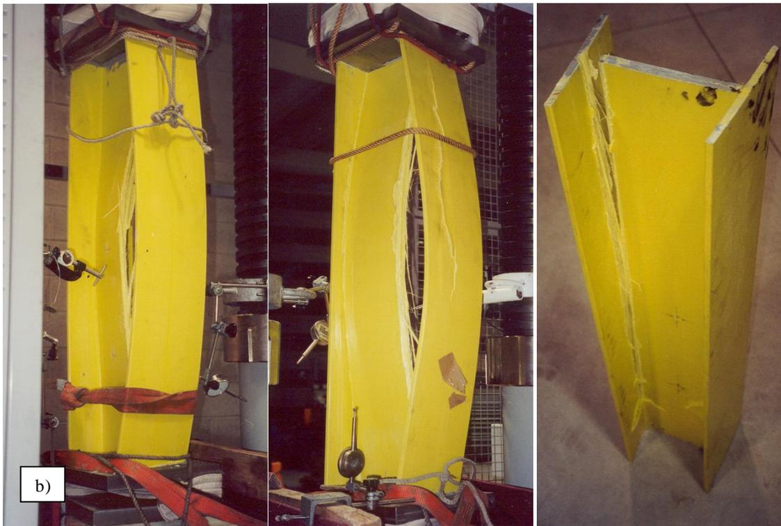
Figure 4. a) Load-axial displacement curve also with lateral displacement curves (coloured and on the left) at the half of the column; b) failure mode. FRP column, "H" shape;  $h=1000\text{ mm}$
