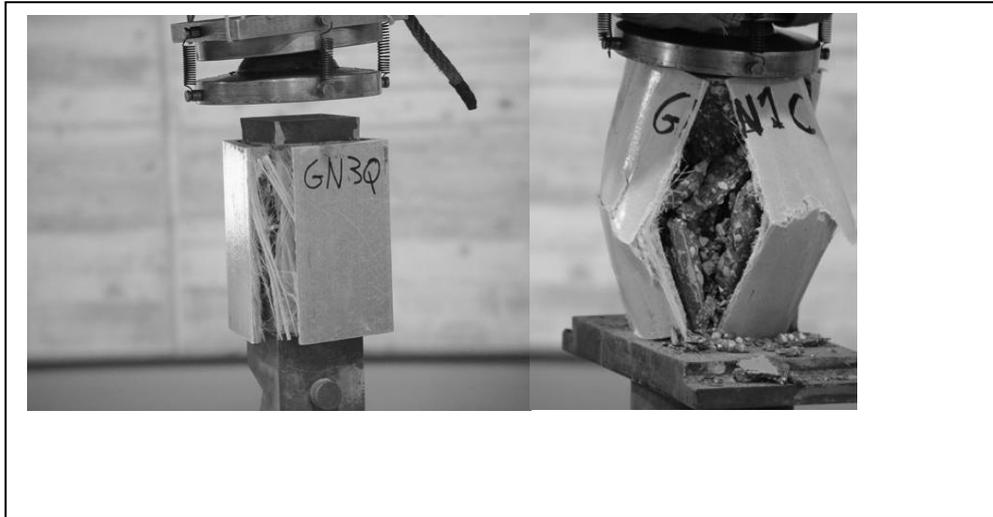
Figure 6. Typical collapses of complex column FRP/Concrete with very low values of  $\lambda$
