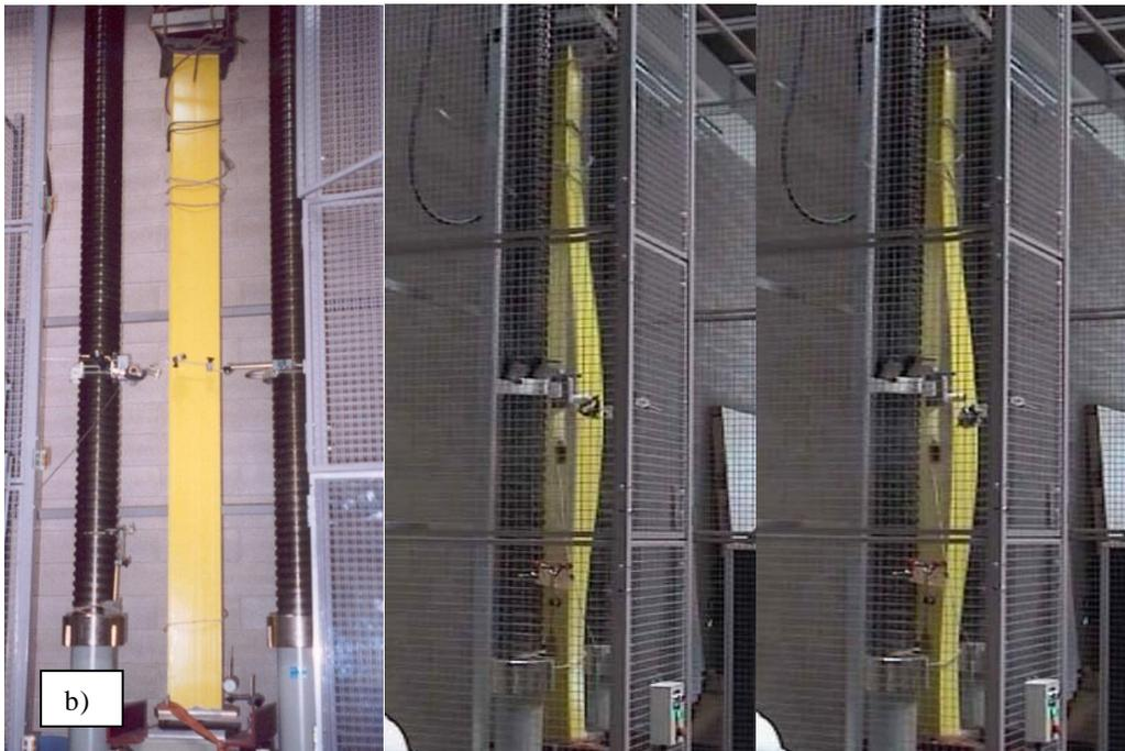
Figure 5. a) Load-axial displacement curve also with lateral displacement curves (coloured and on the left) at the half of the column; b) failure mode. FRP column, "H" shape;  $h = 2800\text{ mm}$
