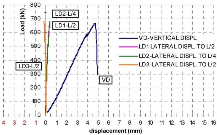
Figure 9. Load-displacement curves, FRP/Concrete, sample  $\lambda = 19.51$
