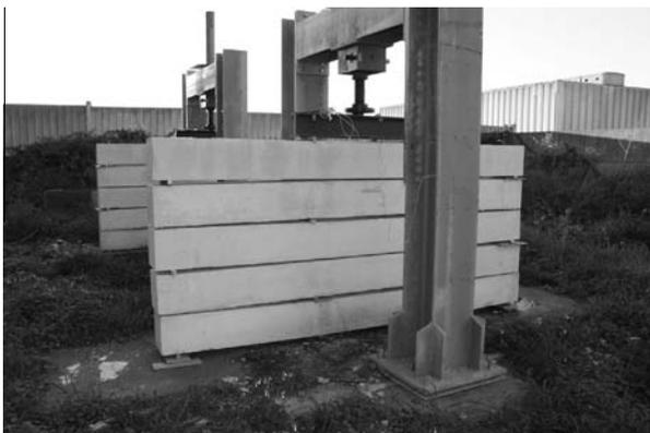
Fig. 1a. Exposed beam under the two loading frames (frame 1 and frame 2).
