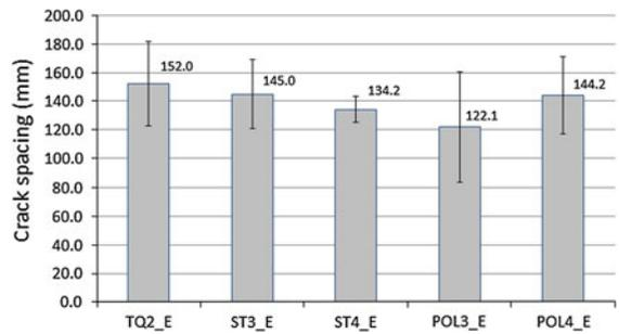
Fig. 9 Average crack spacing between loading points of S1beams of frame 2
