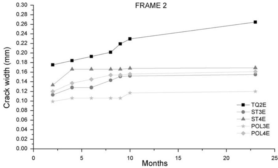
Fig. 5 Average crack width versus time measured on S1 beams of frame 2
