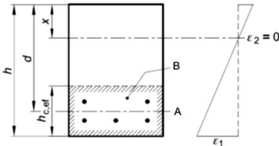
Fig. 13  $A_{ce}$  for RC beams in bending according to EC2
