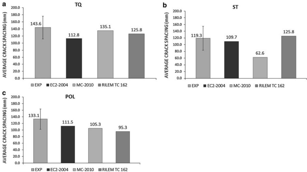
Fig. 14 Comparison between experimental and theoretical average crack spacing of S1 and S2 beams (a TQ beams, b ST beams, c POL beams)
