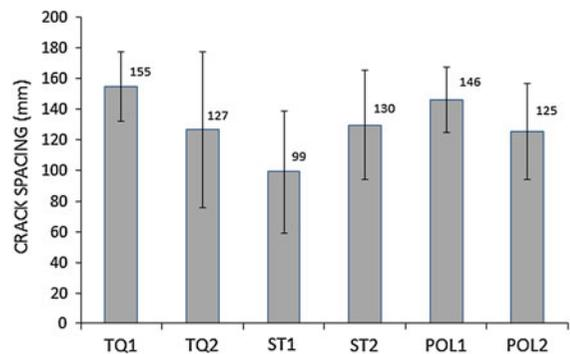
Fig. 12 Average crack spacing of S2 beams
