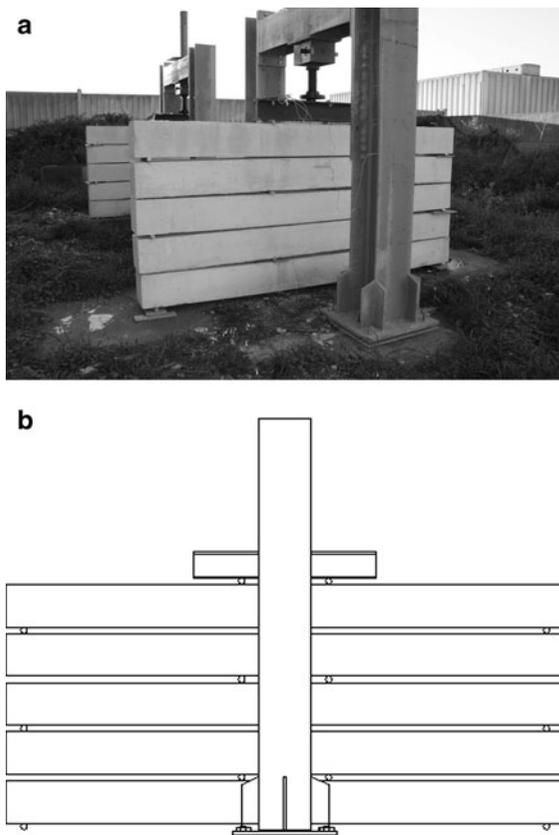
**Fig. 1** a S1 beams under sustained loading. b Details of supports position
