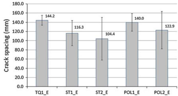
Fig. 8 Average crack spacing between loading points of S1beams of frame 1
