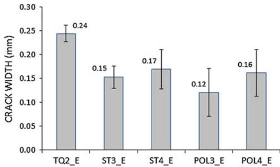
Fig. 7 Average crack width after 17 months of loading (frame2 S1 beams)
