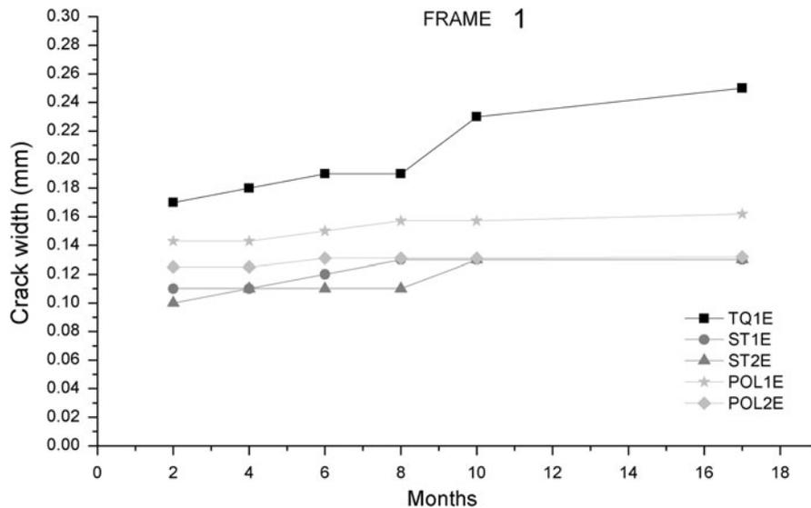
**Fig. 4** Average crack width versus time measured on S1 beams of frame 1
