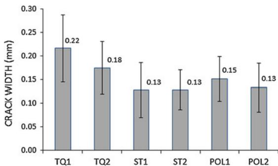
Fig. 11 Average crack width of S2 beams at 50 kN
