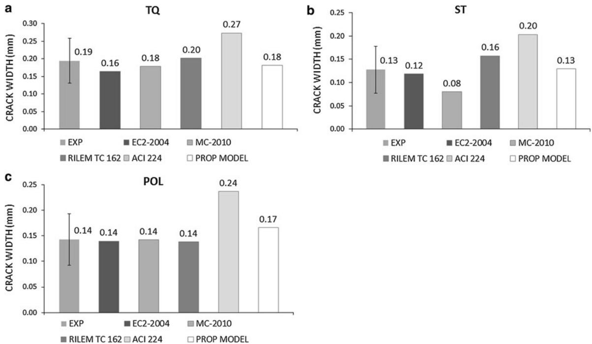
**Fig. 15** Experimental and theoretical crack width of S2 beams (short term loading) (a) TQ beams, (b) ST beams, (c) POL beams)
