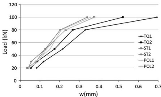
Fig. 10 Load-average crack widths ( $w$ ) curves of S2 beams
