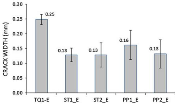
Fig. 6 Average crack width after 17 months of loading (frame1 S1 beams)
