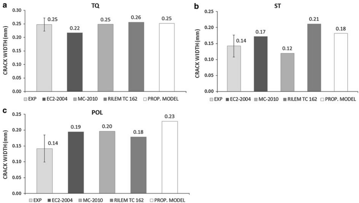
**Fig. 16** Experimental and theoretical crack width of S1 beams (long term loading) (a TQ beams, b ST beams, c POL beams)
