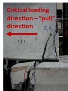
**Fig. 7 – (Left) compressed bar buckling due to plastic hinging over the concrete floor, for loose stirrups [ Protezione Civile 2012]; (right) failure of the zone around the plug for excessive deformation and insufficient stirrups in the support and cover in the beam [Fishinger 2014].**
