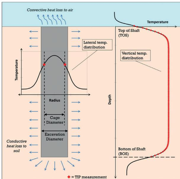
Fig. 2 – Temperature distributions in an idealized shaft. Theoretical radial temperature distribution of shaft cross-section slice (left); theoretical vertical temperature distribution (right).
