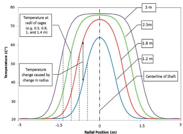
Fig. 3 – Radial temperature distribution for various shaft sizes [MULLINS, 2012].
