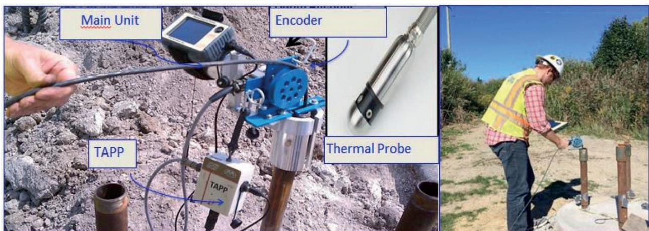
Fig. 5 – Thermic Probe Method (TPM).
