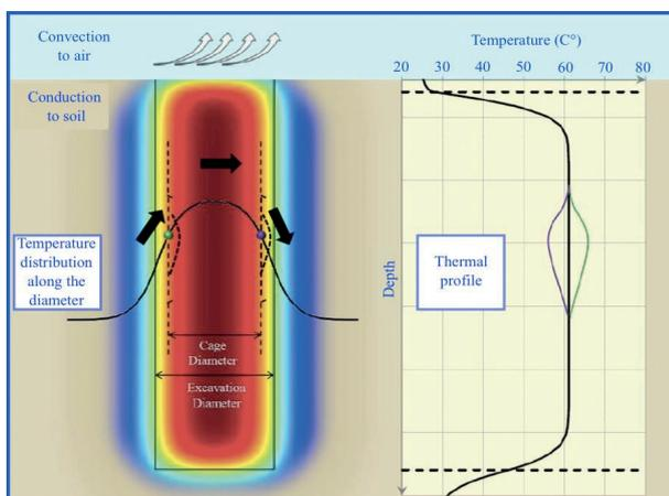
Fig. 9 – Example of reinforcing cage eccentricity.
