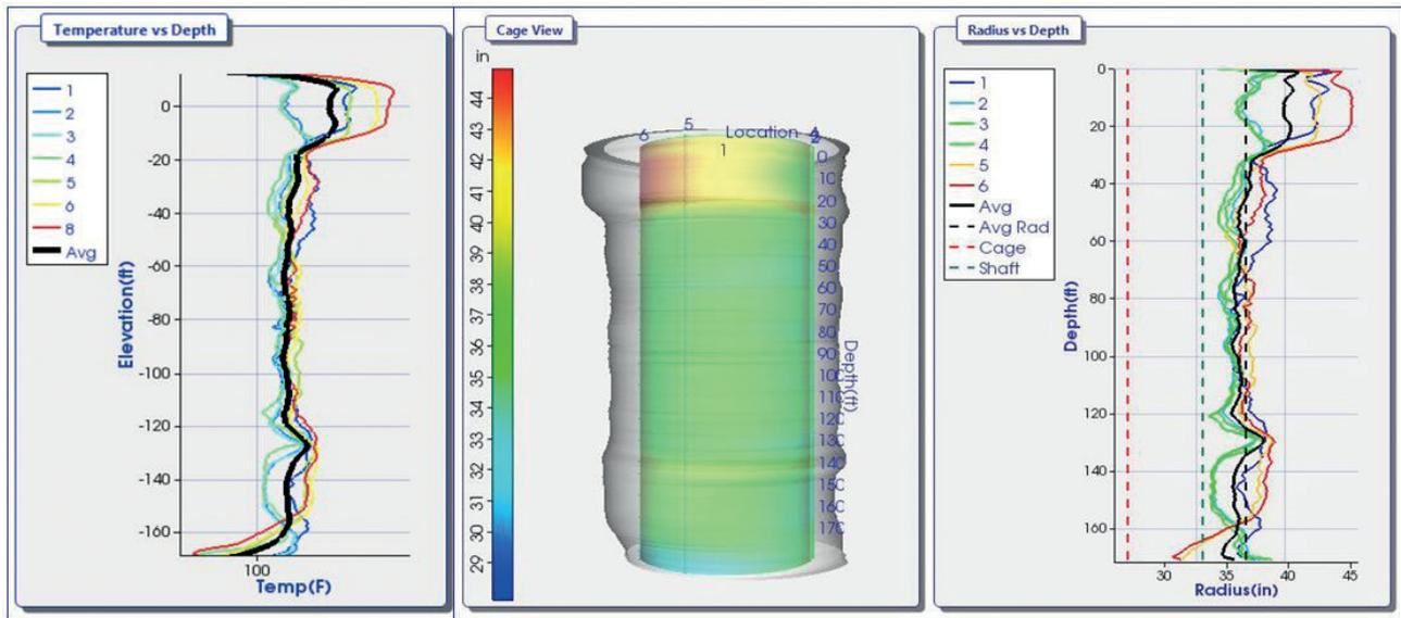
Fig. 12 – TIP testing. Thermal profiles registered (left); shaft shape, model output (center); radius along the shaft axis, as calculated from the software (right).
