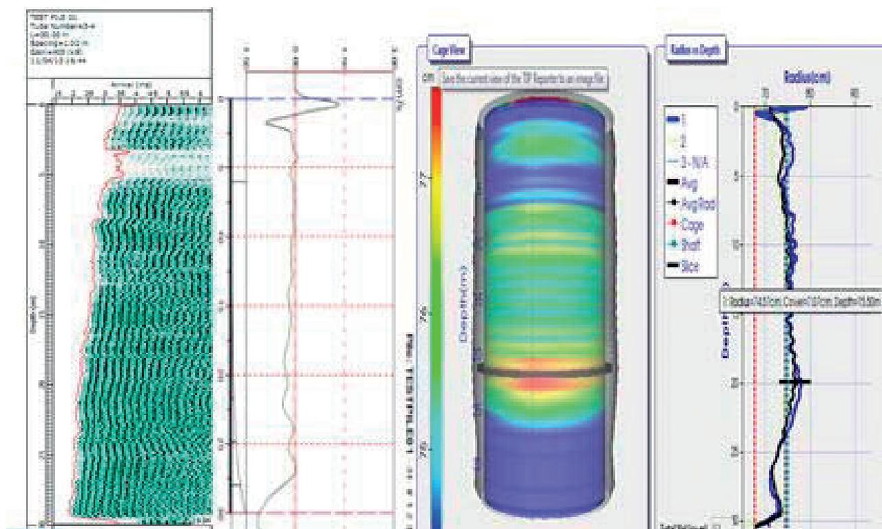
Fig. 13 – Results of the three methods: CSL (left); PIT (center); TIP (right).
