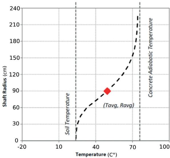
Fig. 4 – Relationship between shaft size and temperature for a given cage position.
