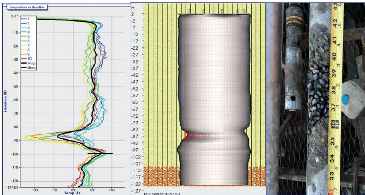
Fig. 7 – Example of necking. Thermal profile registered (left); model output (center); drilling at the anomaly depth (right).
