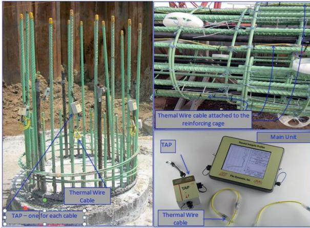
Fig. 6 – Thermal Wire Method (TWM).
