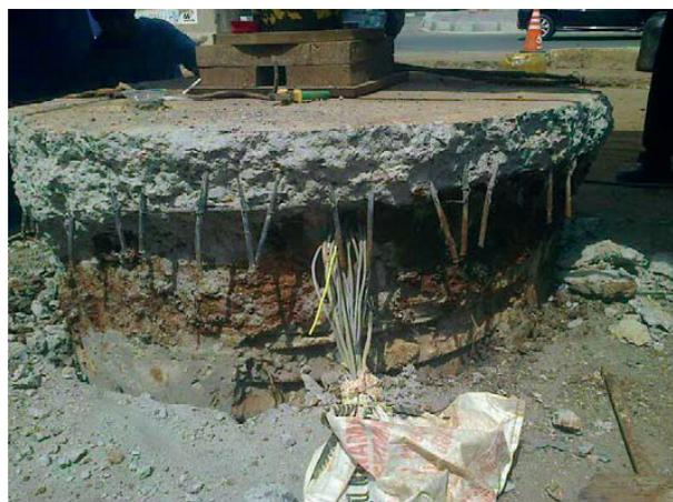
Fig. 14 – Shaft excavated to show the defect identified by the TIP.
