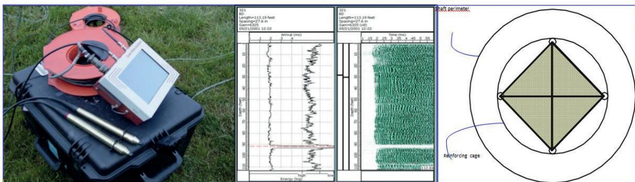
Fig. 10 – Cross-hole equipment; example of testing result; analysed shaft area.
