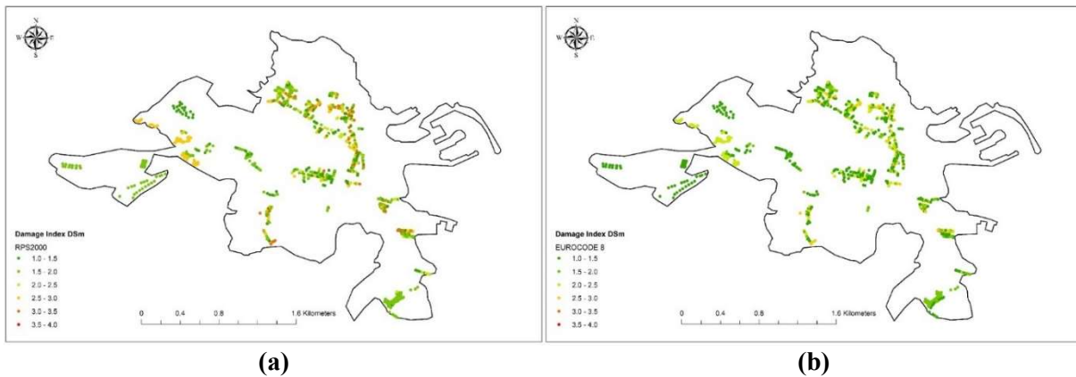
Figure 12: Damage distribution in the city of Al Hoceima, following (a) the RPS2000 risk scenario and (b) the Eurocode 8 risk scenario
