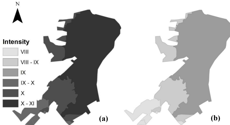
Figure 2: (a) Intensity Map of the City of Imzouren Including Site Effects According to (a) Deterministic Scenario and (b) Probabilistic Scenario
