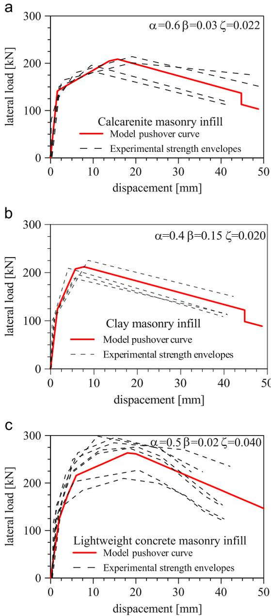
Fig. 23. Calibration of parameters through best pushover-fitting curves. (a) calcarenite masonry infill; (b) clay masonry infill; and (c) lightweight concrete masonry infill.
