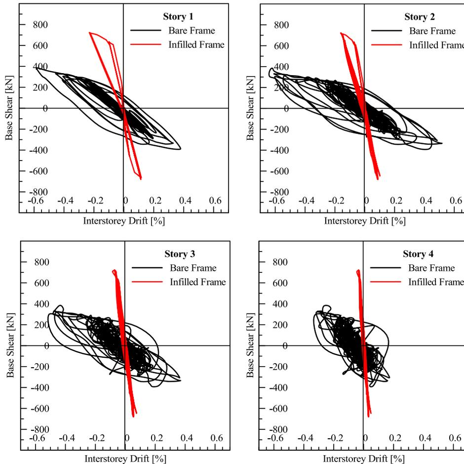
Fig. 39. Infilled and bare frame. Base shear vs. interstorey drift.
