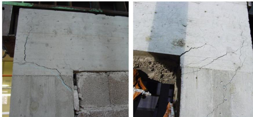
Fig. 15. End of column and beam–column joint damaging.
