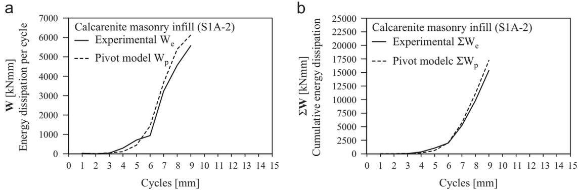
Fig. 30. Experimental/analytical energy dissipation comparison. (a) Energy dissipation per cycle; and (b) Cumulative energy dissipation. S1A-2 specimen.
