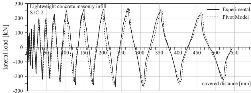
Fig. 29. Experimental/analytical force-lateral covered distance comparison test for a lightweight concrete masonry infilled frame specimen.
