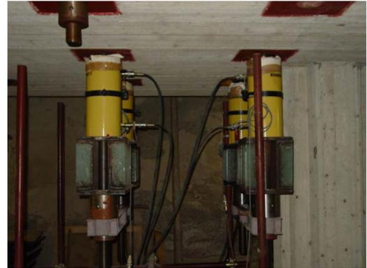
Fig. 6. Hollow hydraulic jacks for vertical load application.
