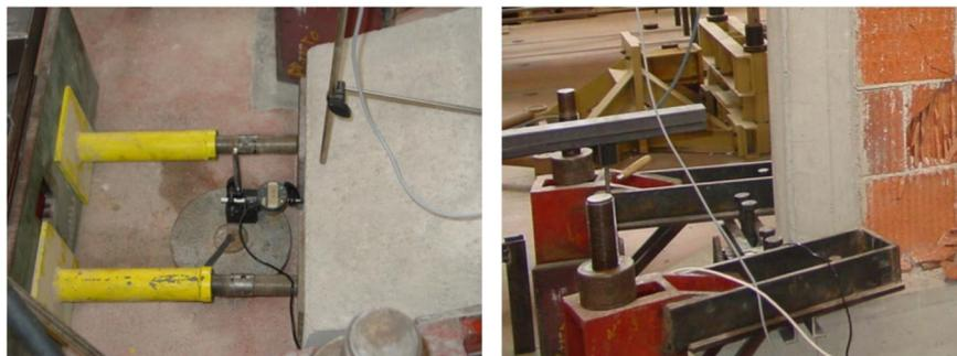
Fig. 8. Specimen translation and rotation constraints.
