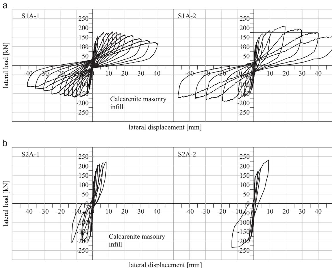
Fig. 12. Force-displacement experimental curves of calcarenite masonry infilled specimens: (a) S1 ; and (b) S2 series.
