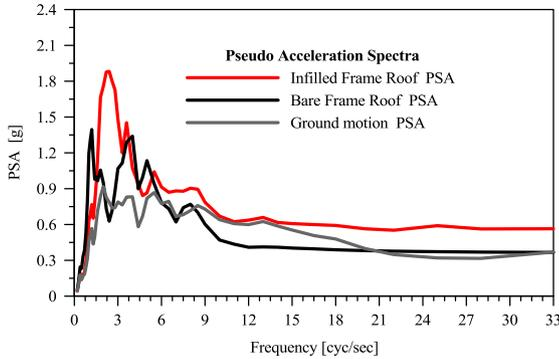
Fig. 38. Pseudo acceleration spectra for ground motion, roof bare frame and roof infilled frame.
