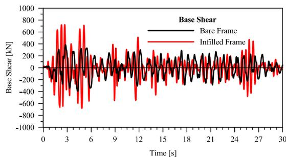
Fig. 35. Infilled and bare frame. Base shear vs. time.
