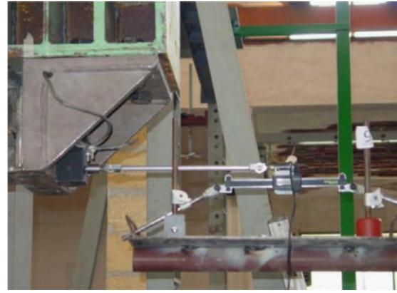
Fig. 9. Transducer for the top lateral displacement measuring.
