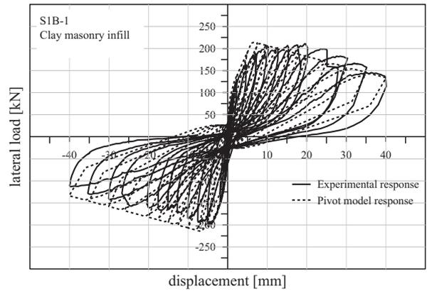
Fig. 25. Experimental/analytical cyclic response for a clay masonry infilled frame specimen.
