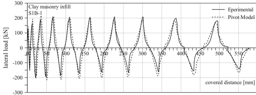
Fig. 28. Experimental/analytical force-lateral covered distance comparison test for a clay masonry infilled frame specimen.
