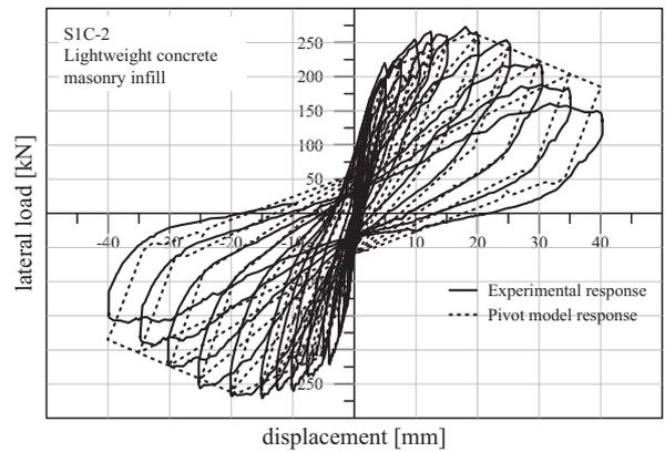
Fig. 26. Experimental/analytical cyclic response of lightweight for a concrete masonry infilled frame specimen.
