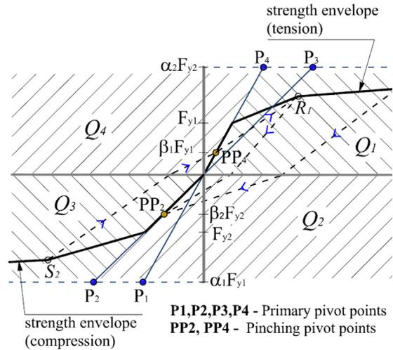
Fig. 18. Hysteretic Pivot model for a generic unsymmetrical tension–compression law.
