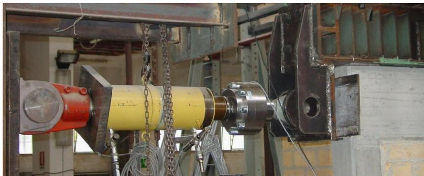
Fig. 7. Hydraulic jack for lateral load application.
