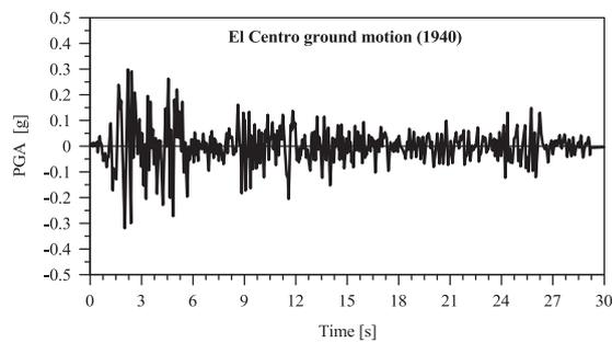
Fig. 34. Ground motion record used for the analyses (El Centro, 1940).
