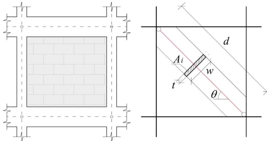
Fig. 1. Equivalent diagonal single strut definition and geometrical characteristics.
