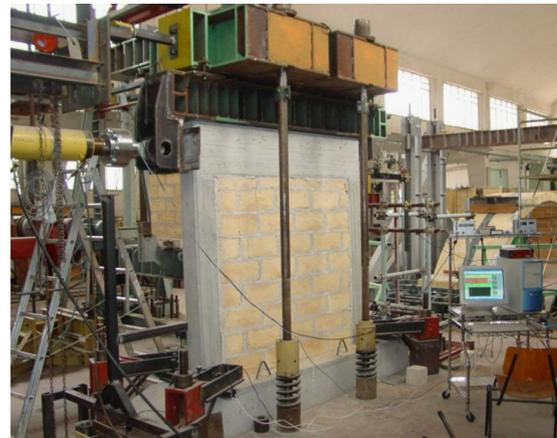
Fig. 10. A specimen in the test apparatus.
