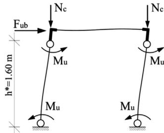
Fig. 11. Simplified scheme for the evaluation of the lateral strength of bare frames.
