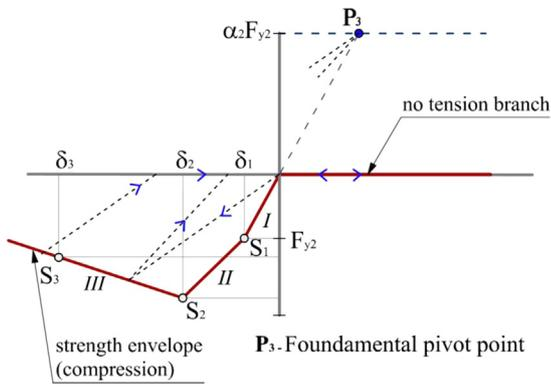
Fig. 19. Hysteretic Pivot law particularization for the equivalent diagonal strut.
