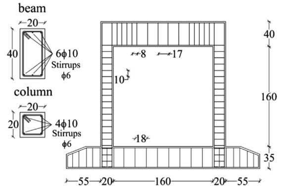
Fig. 2. S1A and S1B specimen details (measures in cm).
