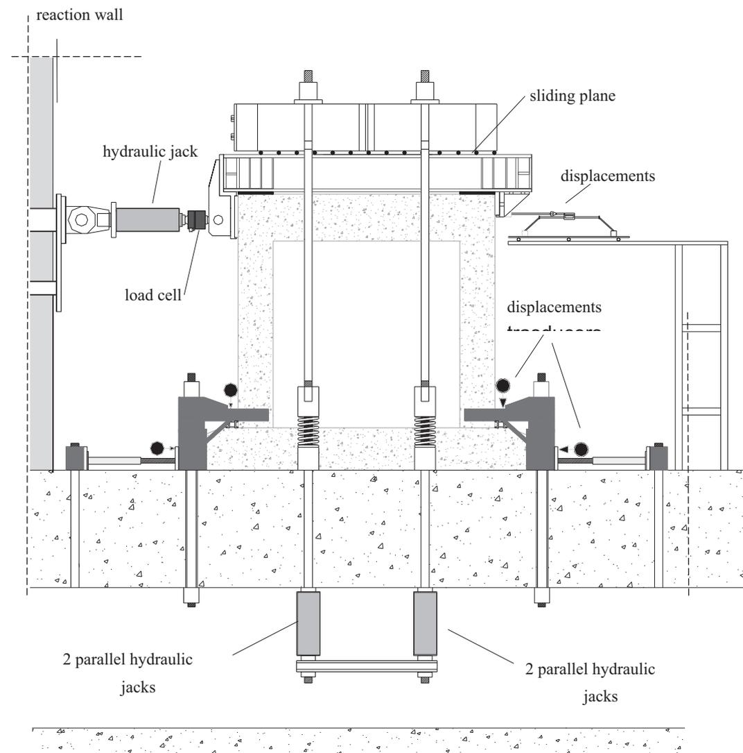
Fig. 5. Test set up.
