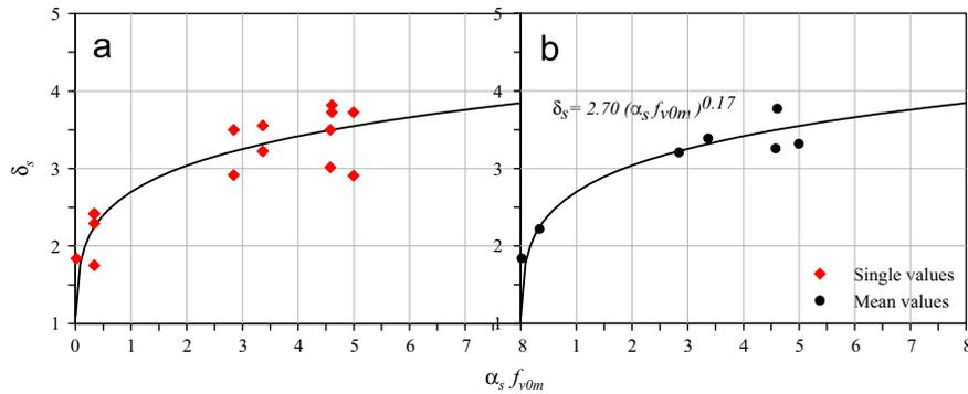
Fig. 17.  $\delta_s$ - $\alpha_s f_{v0m}$  correlation: (a) values of  $\delta_s$  referred to each specimen; and (b) mean values of  $\delta_s$  referred to each typology of specimens.
