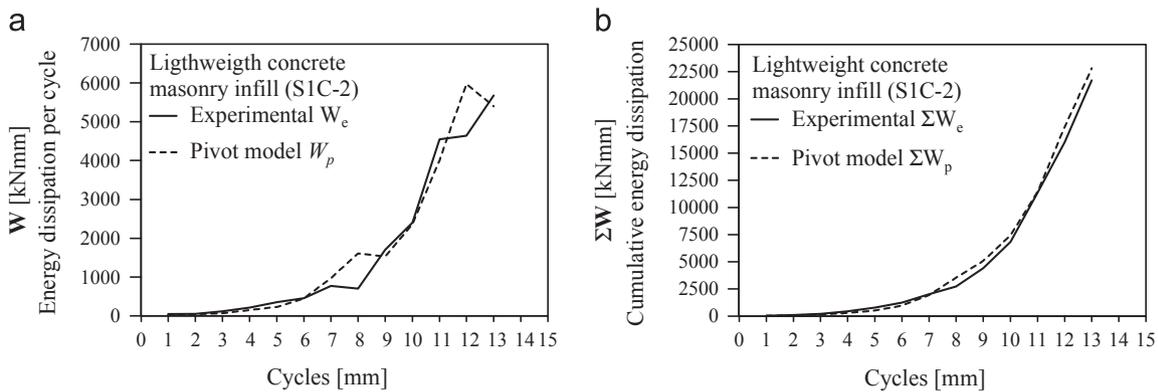
Fig. 32. Experimental/analytical energy dissipation comparison. (a) Energy dissipation per cycle; and (b) Cumulative energy dissipation. S1C-2 specimen.
