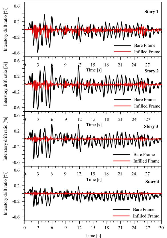
Fig. 37. Infilled and bare frame. Interstorey drifts.
