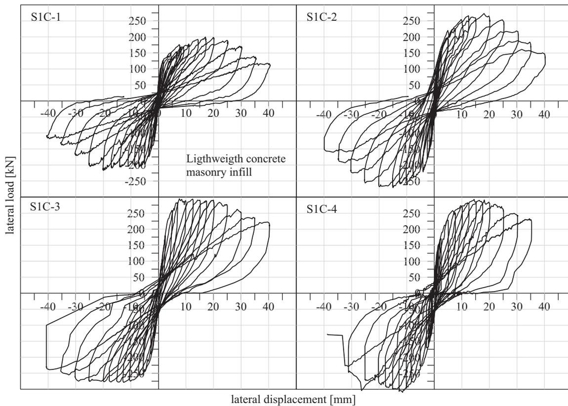
Fig. 14. Force–displacement cyclical test results for lightweight concrete infilled specimens. S1 series.
