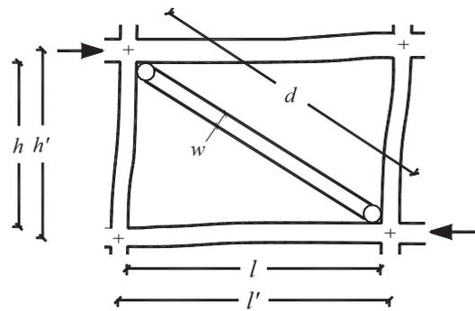
Fig. 21. Geometrical features of frame with strut equivalent to infill.
