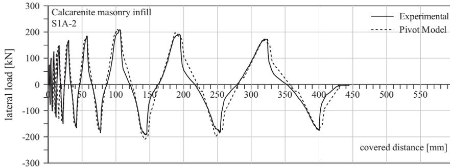
Fig. 27. Experimental/analytical force-lateral covered distance comparison test for a calcarenite masonry infilled frame specimen.
