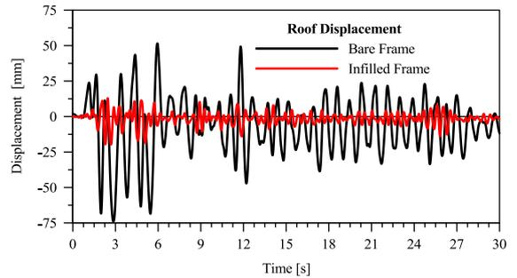
Fig. 36. Infilled and bare frame. Roof displacement vs. time.
