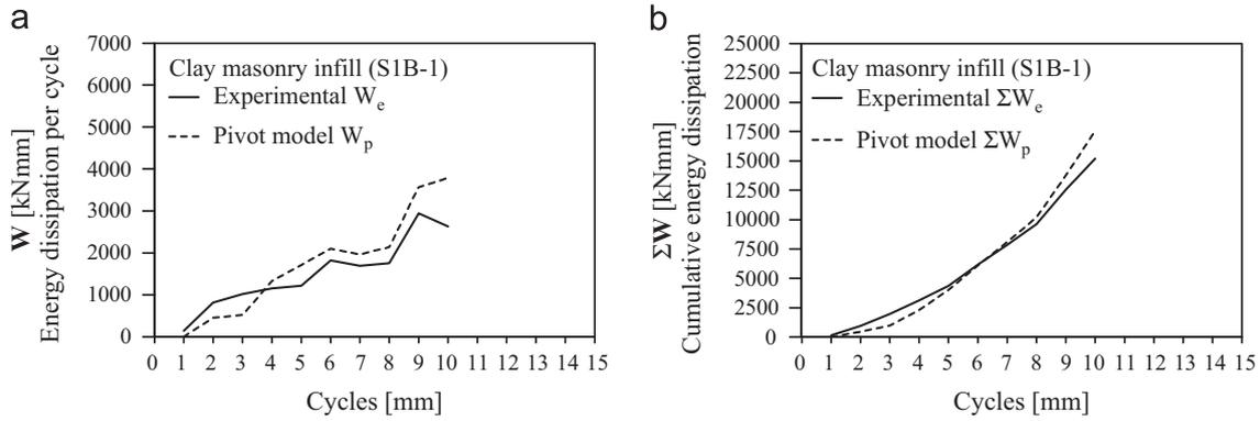
Fig. 31. Experimental/analytical energy dissipation comparison. (a) Energy dissipation per cycle; and (b) Cumulative energy dissipation. S1B-1 specimen.
