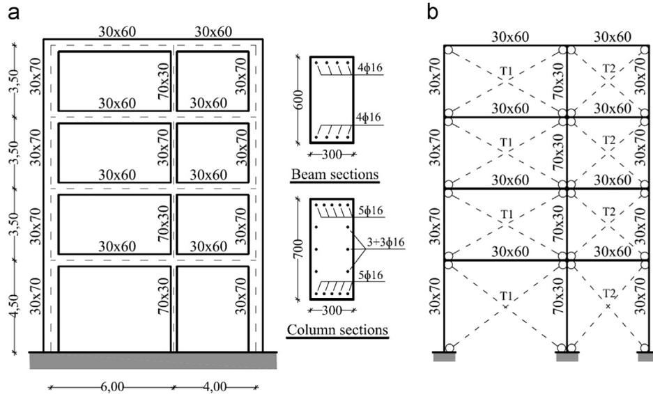
Fig. 33. Prototype structure. (a) geometry and cross section features; and (b) model of the infilled/bare frame.
