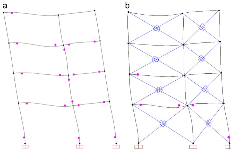
Fig. 40. Hinges yielding at the end of the ground motion. (a) bare frame; and (b) infilled frame.
