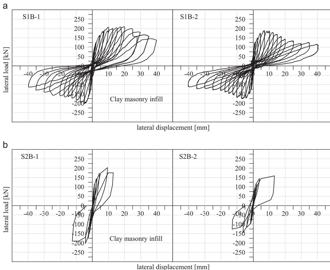
Fig. 13. Force–displacement experimental curves of clay masonry infilled specimens: (a) S1 ; and (b) S2 series.
