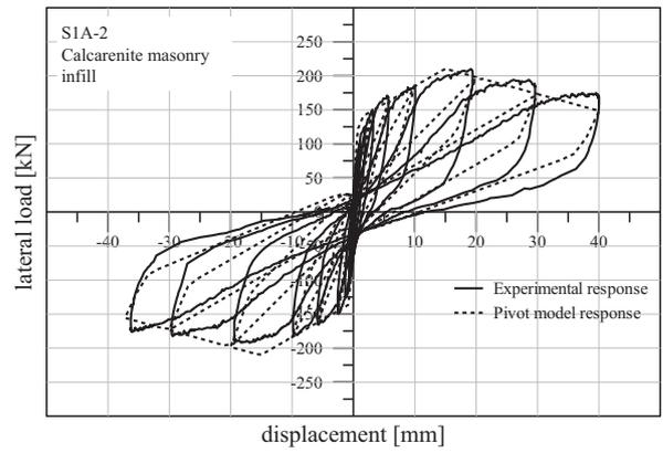
Fig. 24. Experimental/analytical cyclic response for a calcarenite masonry infilled frame specimen.
