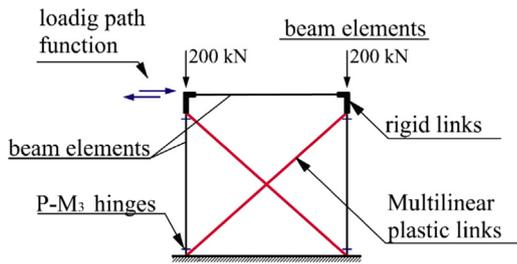
Fig. 20. Structural FEM model employed for the analyses.
