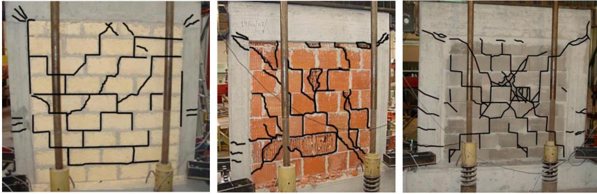
Fig. 16. Typical specimen cracking patterns at the end of the tests.
