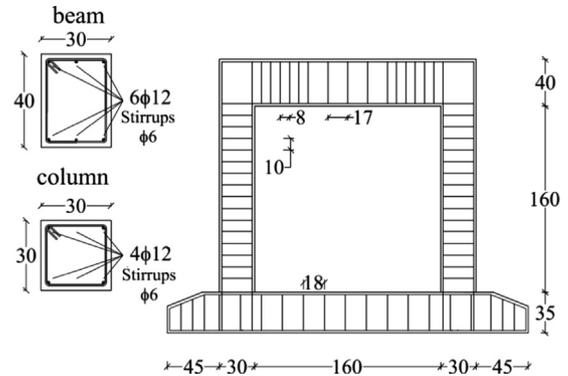
Fig. 3. S1C specimen details (measures in cm).
