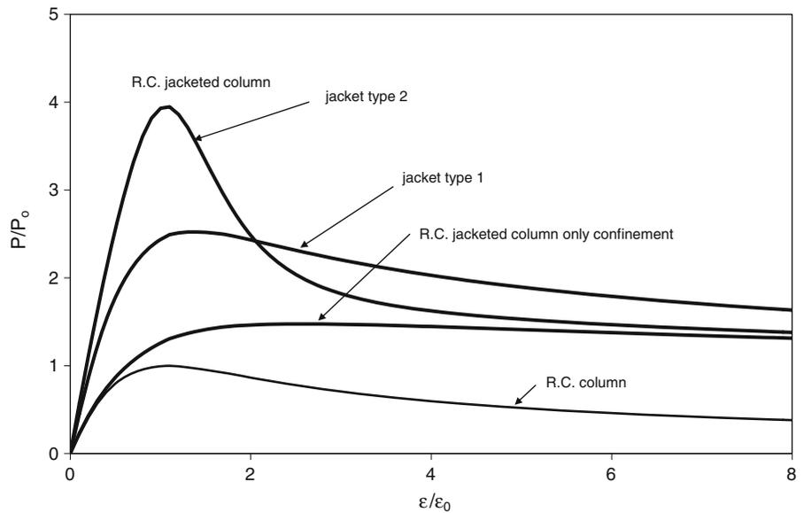
**Fig. 13** Effect of thickness of concrete jacket on moment axial force domain
