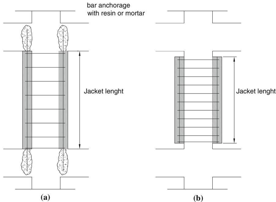
**Fig. 1** Concrete jacketing techniques; **a** jacket directly loaded; **b** jacket indirectly loaded
