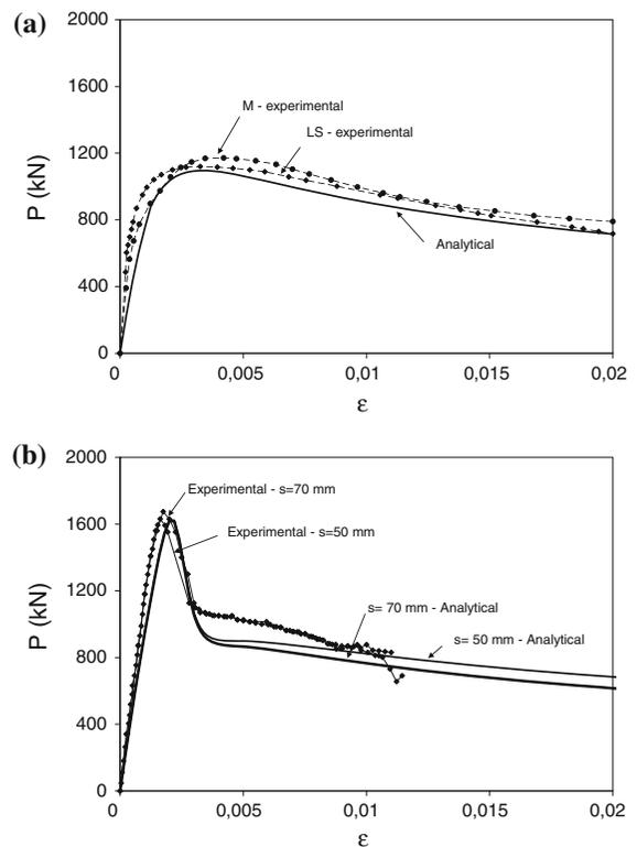
**Fig. 9** Comparison of experimental results (load shortening curve) and analytical prediction obtained with the proposed model: **a** data of Ersoy et al. [9]; **b** data of Takeuti et al. [21]
