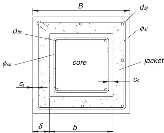
Fig. 2 RC columns externally jacketed
