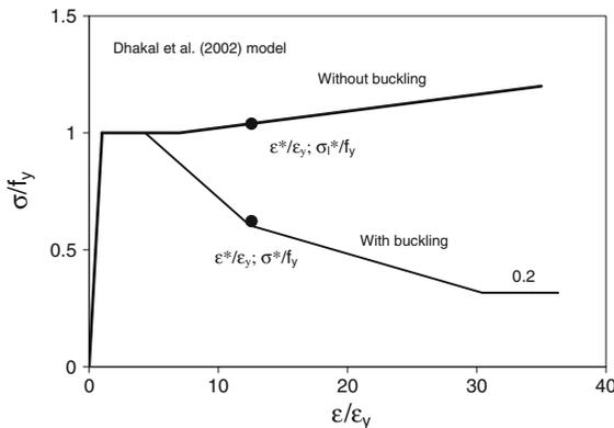
**Fig. 7** Stress–strain curves adopted for compressed bars according to Dhakal et al. (2002)
