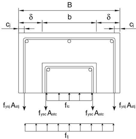
**Fig. 3** Equilibrium of the transverse cross-section and calculation of confinement pressure
