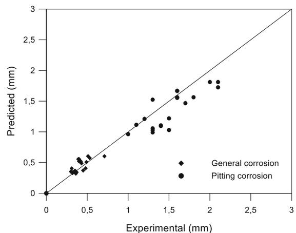
**Fig. 4** Experimental versus theoretical reduction in bar section
