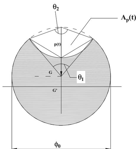
**Fig. 3** Pitting attack in a reinforcing bar according to the model given in [4]
