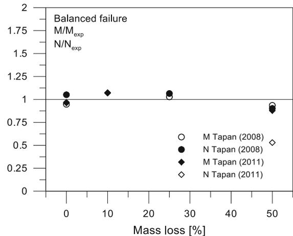
**Fig. 13** Comparison between analytical and experimental ultimate axial force bending moment
