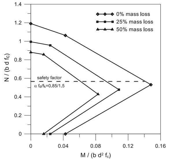
**Fig. 15** Dimensionless diagram of axial force-bending moment versus loss of mass
