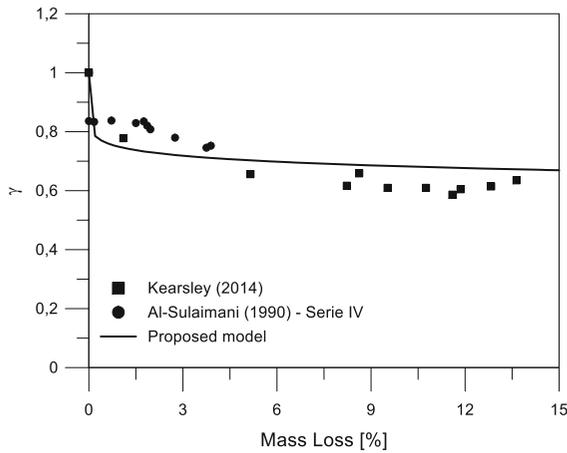
**Fig. 7** Experimental versus theoretical dimensionless bond strength reduction
