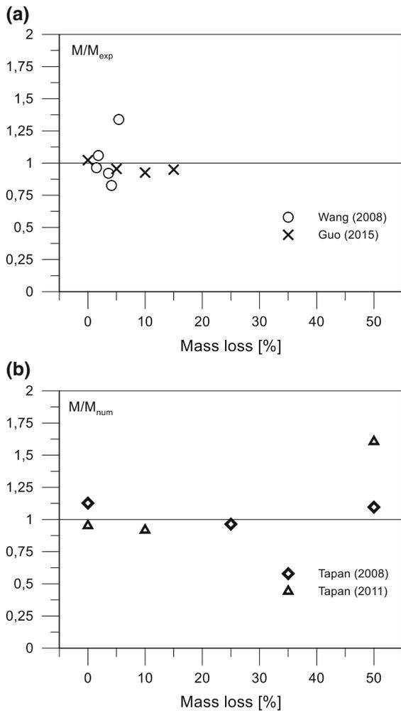
**Fig. 12** Comparison between analytical and **a** experimental ultimate bending moment **b** numerical ultimate bending moment
