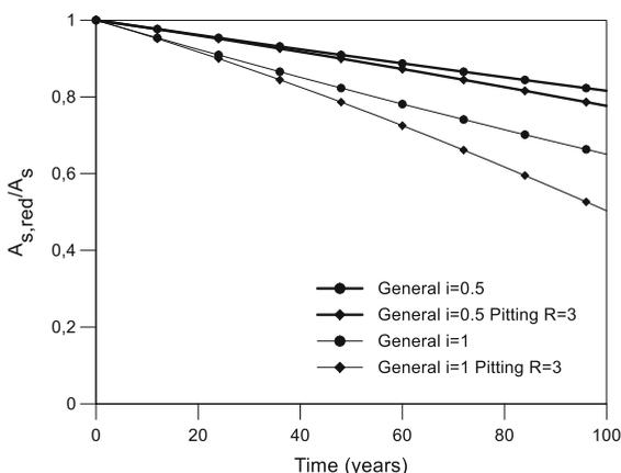
Fig. 5 Normalized reduction of steel area with time increase
