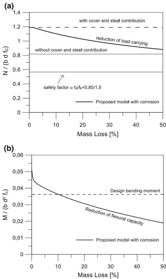
**Fig. 14** Dimensionless diagram of: **a** axial forces versus loss of mass; **b** bending moment versus loss of mass
