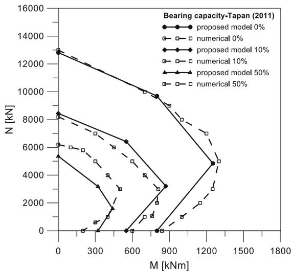
**Fig. 10** Comparison between analytical and experimental interaction diagrams
