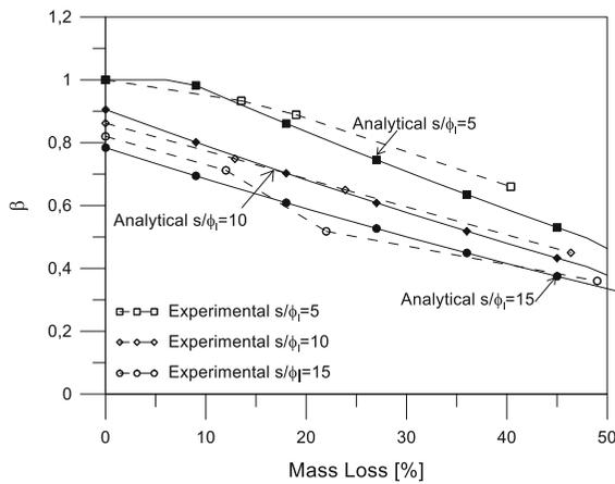
**Fig. 6** Normalized reduction of yielding stress in compressed bar with loss of mass in %
