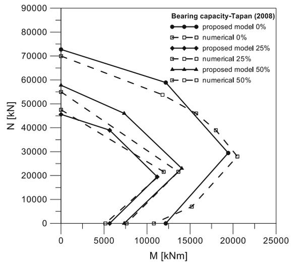
Fig. 9 Comparison between analytical and experimental interaction diagrams
