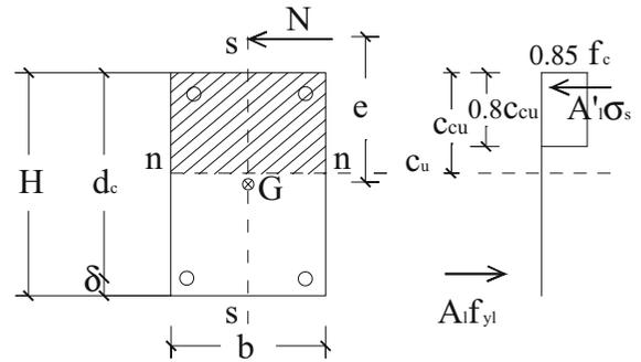
**Fig. 8** Design assumptions for analysis of single R.C. column
