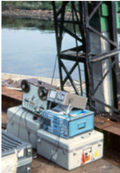
Pile Driving Analyser in 1980 and in PDA-PAX 2010 with wireless sensors
