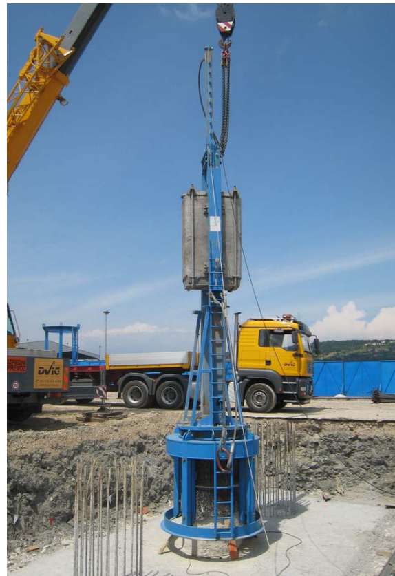
Dynamic Load Test on non-driven piles with 4 ton and 11 ton free fall hammer
