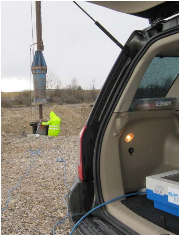
Dynamic Load Test on non-driven piles with 4 ton and 11 ton free fall hammer
