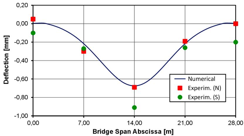
**Figure 15.a** – Deflection comparison for the crown loading (S = South lane, N = North lane)
