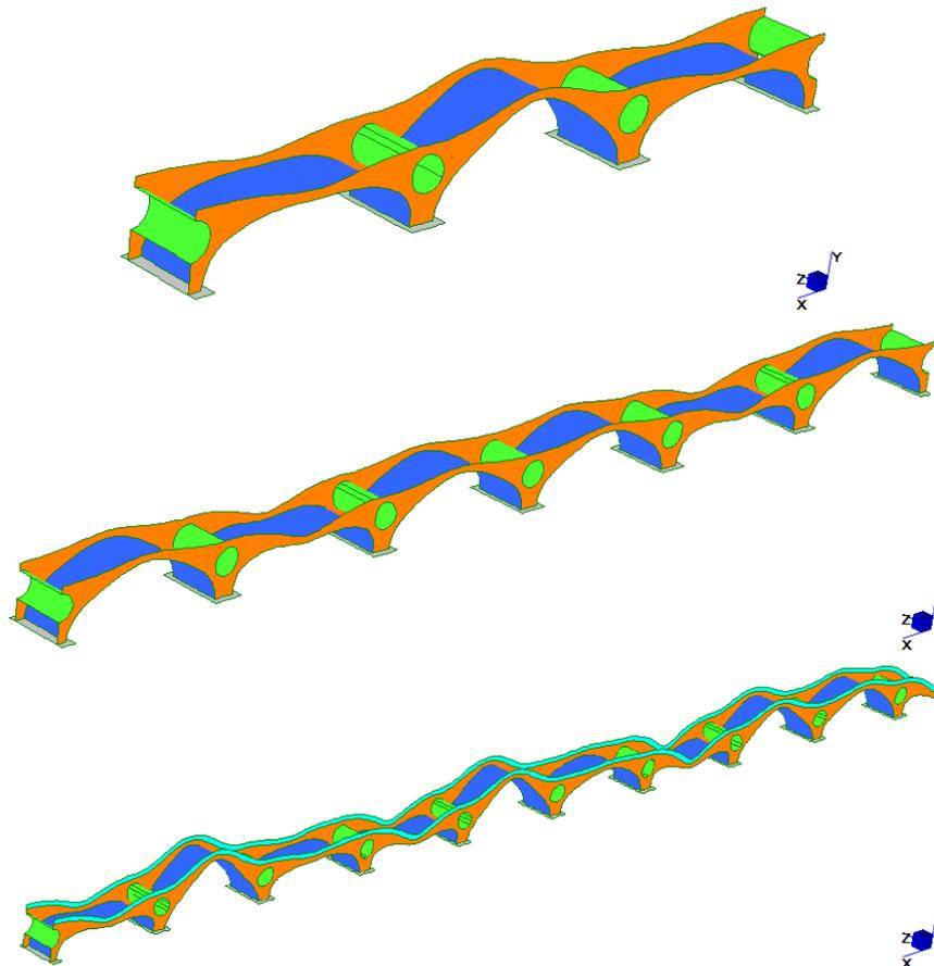
Figure 17 – The three modes with alternating hogging arches: 8.85 Hz approximately
