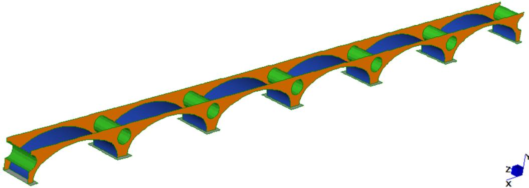
**Figure 13.b** – View of the model composed of six spans of the bridge (fill removed)
