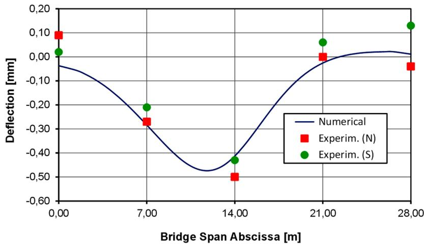
**Figure 15.b** – Deflection comparison for the loading at the arch quarter
