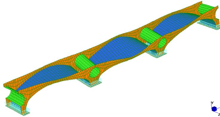
**Figure 14.a** – Transversal torsional-flexural mode, 6,82 Hz
