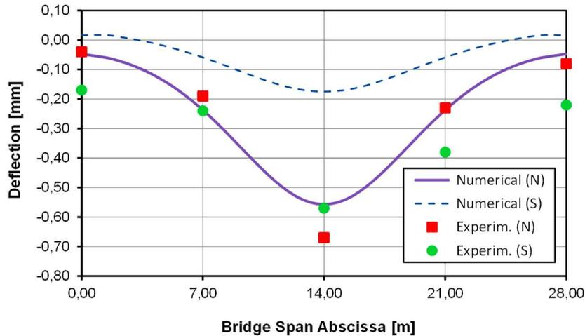
Figure 15.c – Deflection comparison for the line loading on one bridge lane
