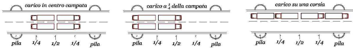
Fig. 11 – Truck arrangement for the static load testing of the bridge
