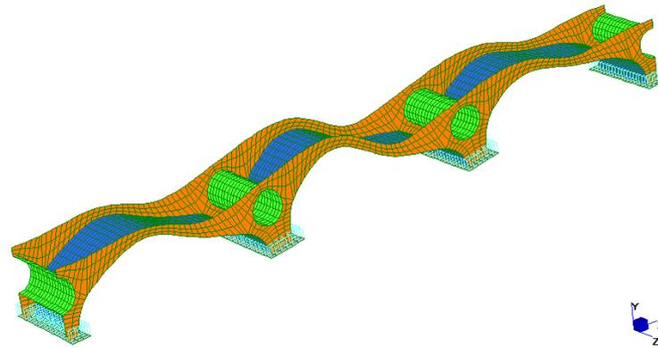
**Figure 14.b** – vertical flexural skew symmetric mode, 7,76 Hz
