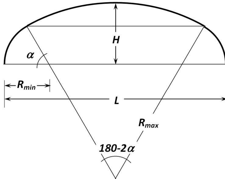
Figure 6 – Polycentric circle segments forming the Perronet Arch
