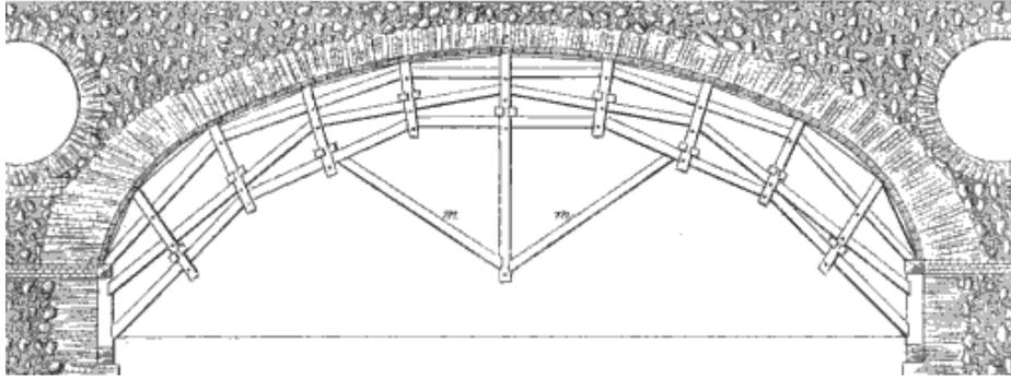
**Figure 2** – Scaffolding proposed by Cavalieri San-Bartolo in the construction of a polycentric arch
