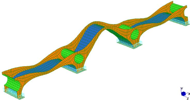
**Figure 14.c** – vertical flexural symmetric mode, 8,78 Hz
