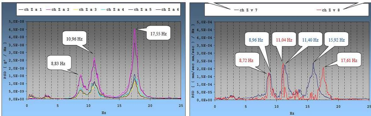
10 – PSD of the signals recorded in “z” vertical direction
