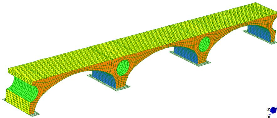
Figure 13.a – View of the model composed of three spans of the bridge (in yellow the fill)
