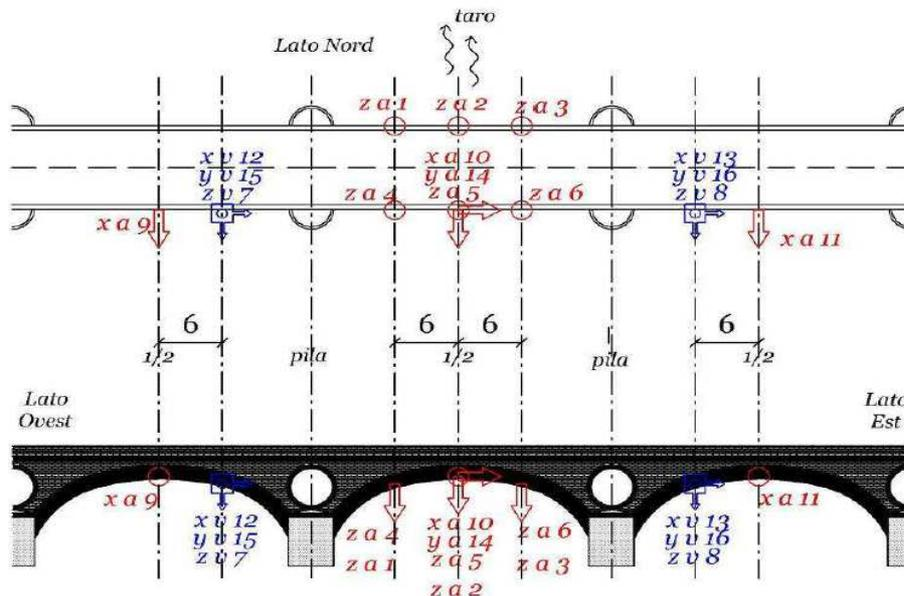
Figure 8 – Position of the accelerometers (a) and seismometers (v); the three indices x, y, and z point out the measurement directions (transversal, longitudinal, vertical)
