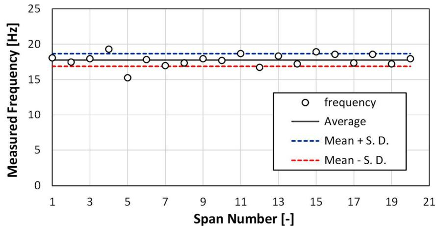
**Figure 18** – Comparison of the selected frequency for the 20 bridge spans
