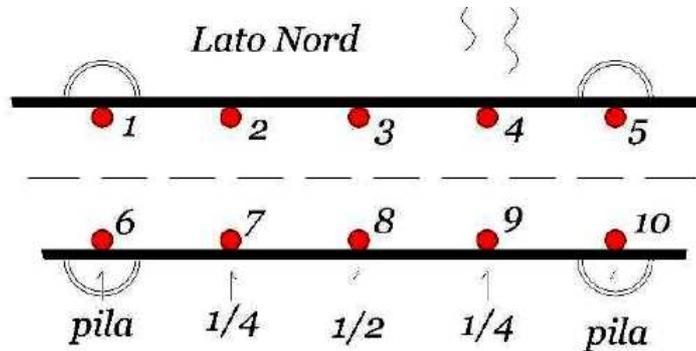
Figure 7 – Instrumented points for the static loading test
