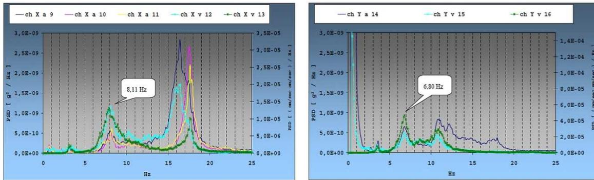
Figure 9 – PSD of the signals recorded in “x” transversal direction and in “y” longitudinal direction
