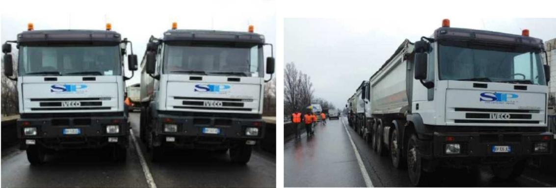
Fig. 12 – View of the trucks over the bridge road for the static tests
