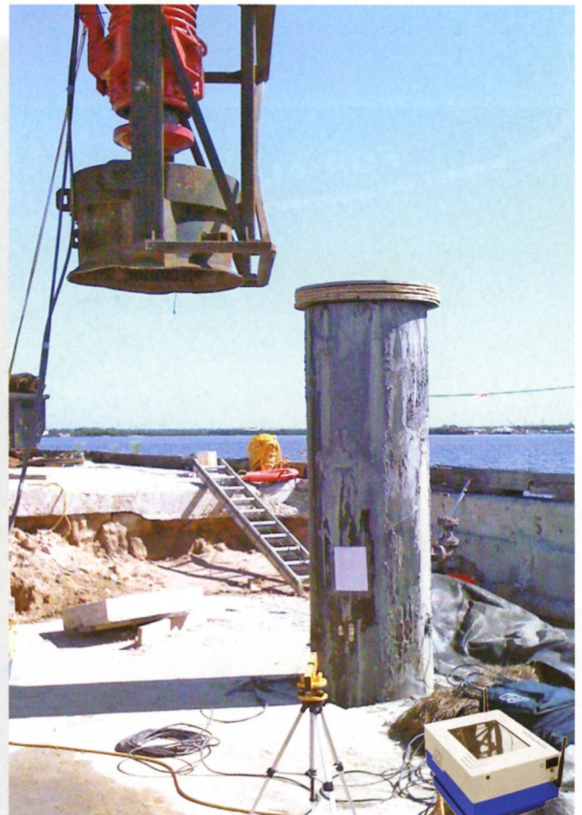
Figure 3: Shaft and PDA testing equipment.
