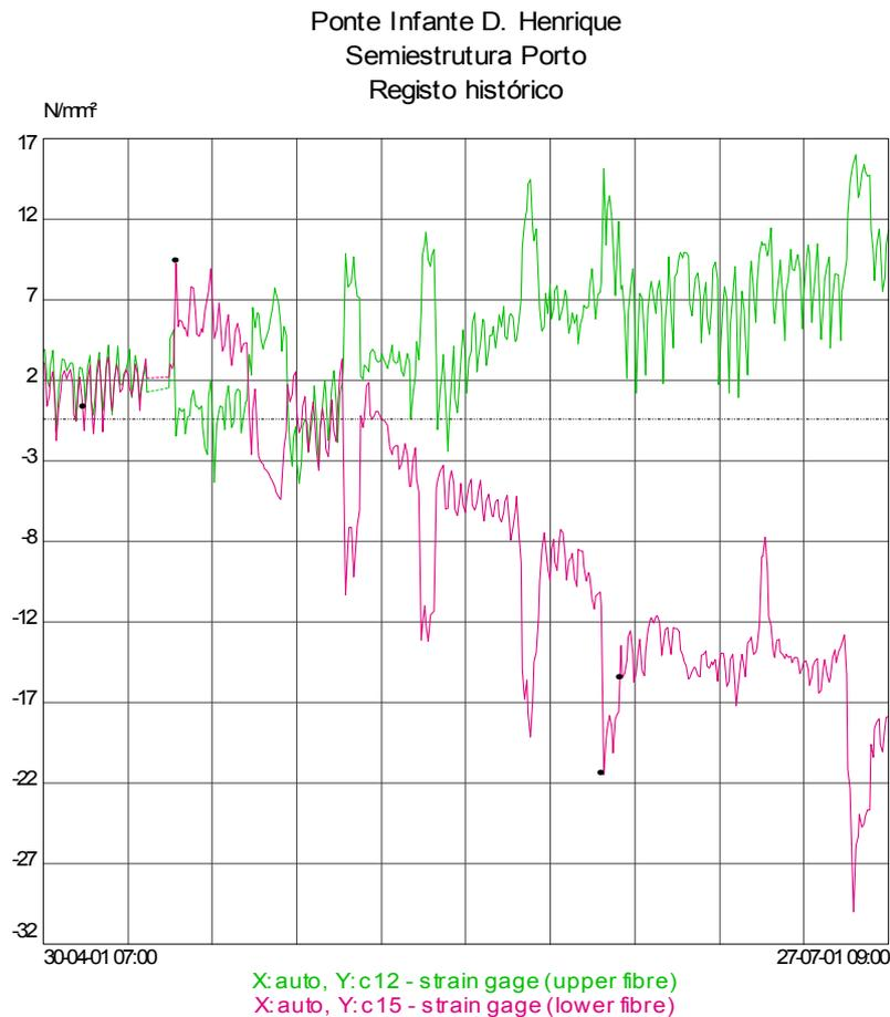
Figure 25 – Development of strains in the upper and lower fibres of the spring cross section of the arch
