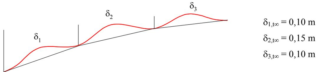
Figure 18 – Definition of the cambers of each half arch
