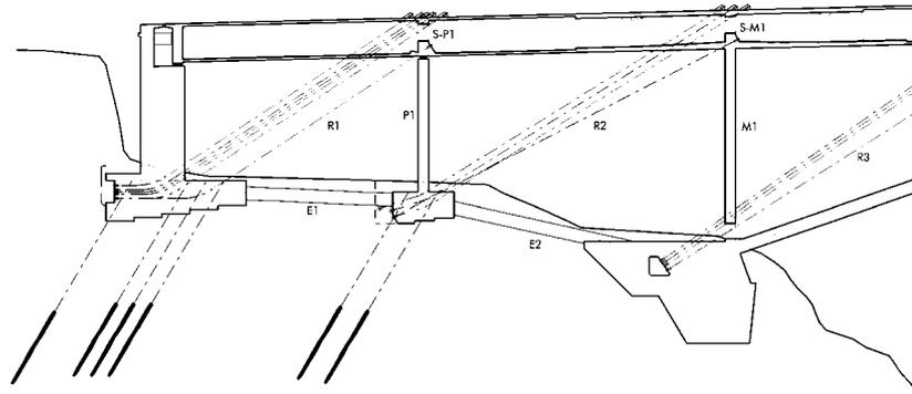
Figure 10 – Backstays, ground struts and anchorages on the Gaia side of the river
