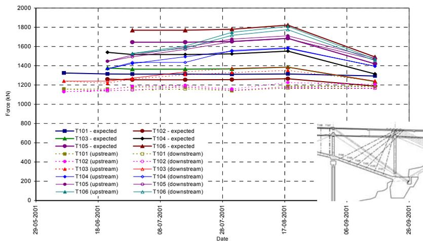
Figure 30 – Variation of axial force on suspension cables of the arch (measured *versus* expected).
