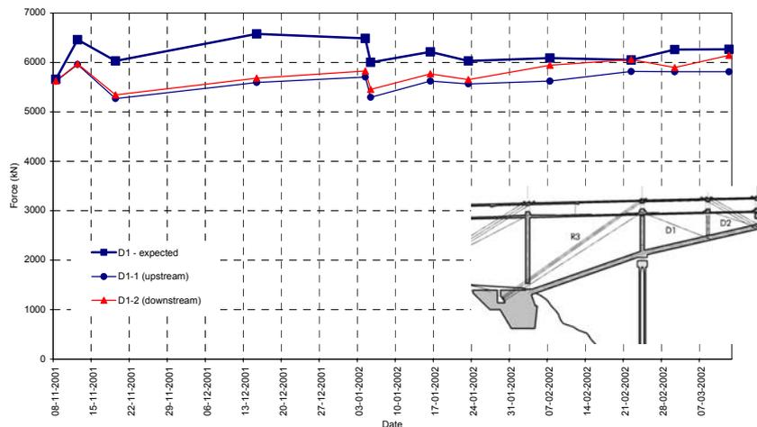
Figure 32 – Variation of axial force on diagonal cable D1 (measured *versus* expected).
