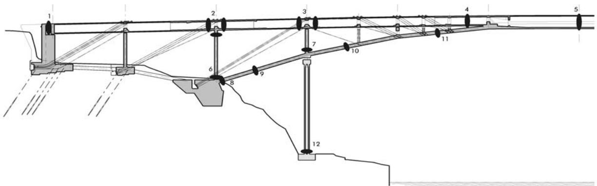
Figure 23 – Location of the sections containing instrumentation in the Gaia half bridge
