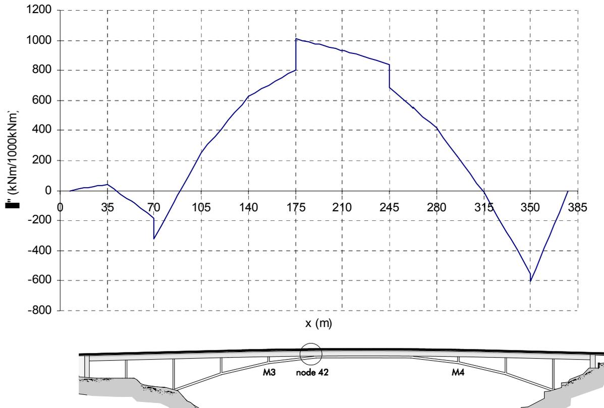
Figure 7 – Coefficient of influence at node 42 of the central span
