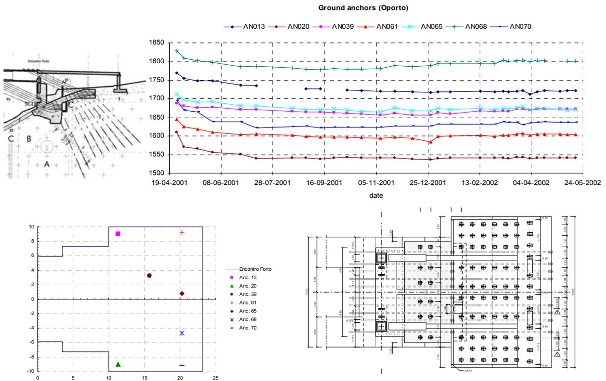
Figure 22 – Location and evolution of forces in monitored ground anchorages in the Oporto side
