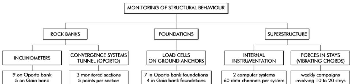
Figure 20 – Monitoring system implemented during construction
