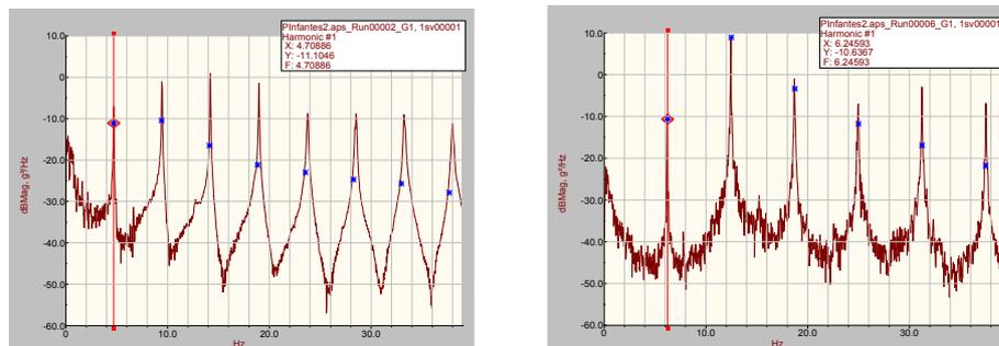
Figure 29 – Average spectral estimates of the ambient response of one suspension cable of the arch during two distinct stages of tensioning.
