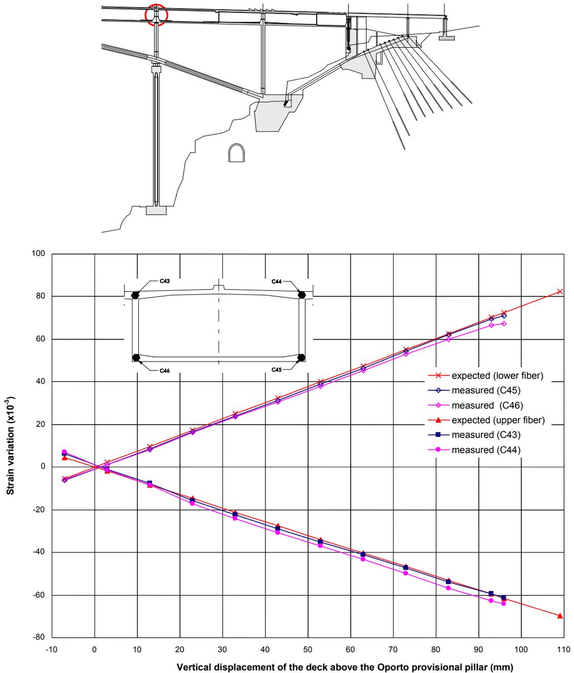
Figure 26 – Strains in the deck cross section above the Oporto provisional pillar
