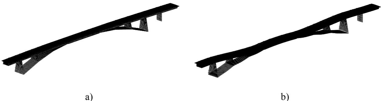
Figura 5 – a) Finite element shell model; b) Deformed bridge under dead weight
