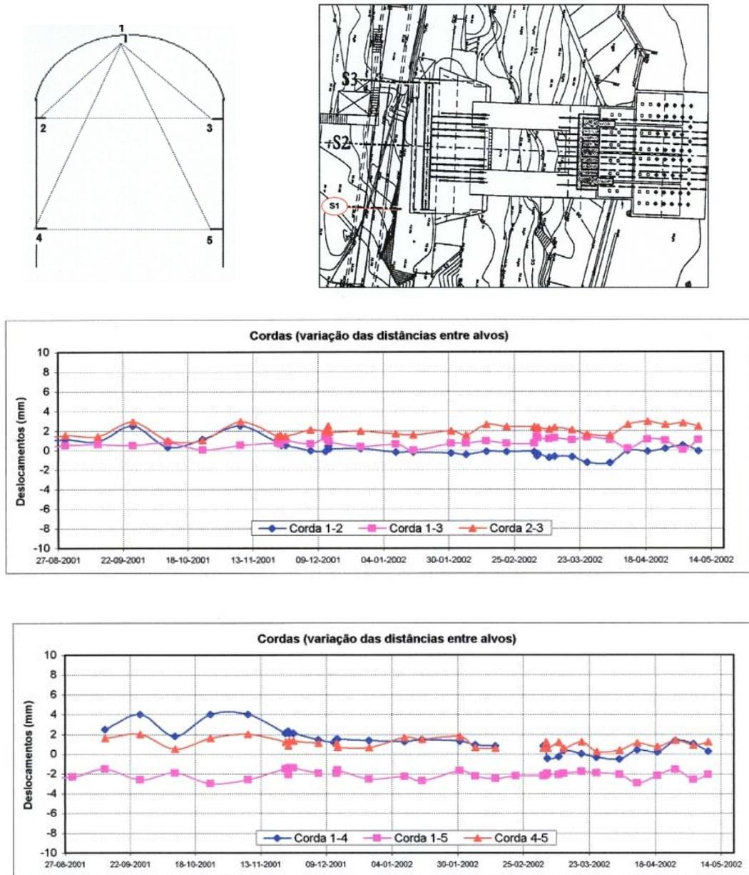
Figure 21 – Optic convergence system in the old tunnel
