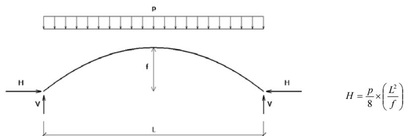
Figure 4 – Structural response of a “perfect arch”
