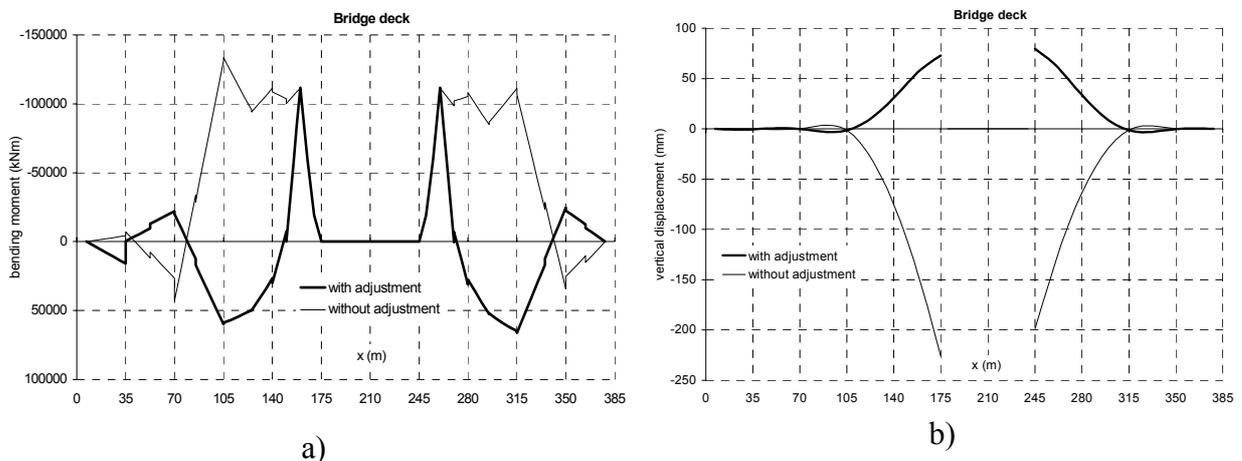
Figure 17 – a) Bending moment diagrams; b) Vertical displacement diagrams
