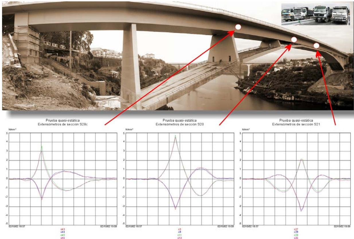
Figure 27 – Lines of influence of strains in three cross sections of the deck
