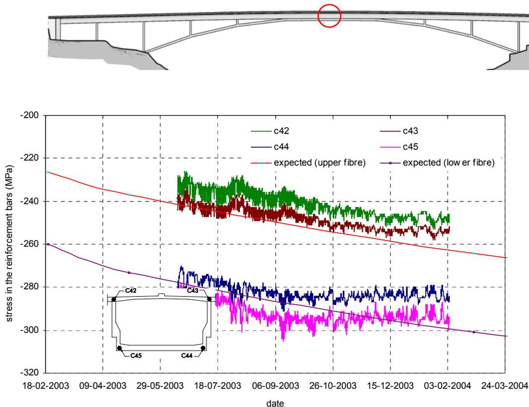
Figure 33 – Stresses in the reinforcement bars at the central cross section of the bridge
