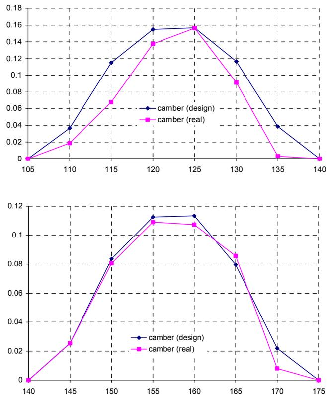
Figure 19 – Comparison between the designed and real cambers
