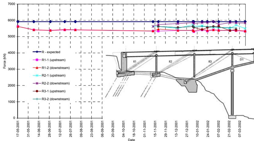
Figure 31 – Variation of axial force on backstay cables R1, R2 and R3 (measured *versus* expected).
