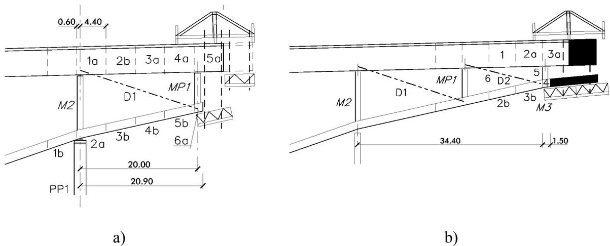
Figure 12 – a) D1 - provisional diagonal; b) D2 - provisional diagonal
