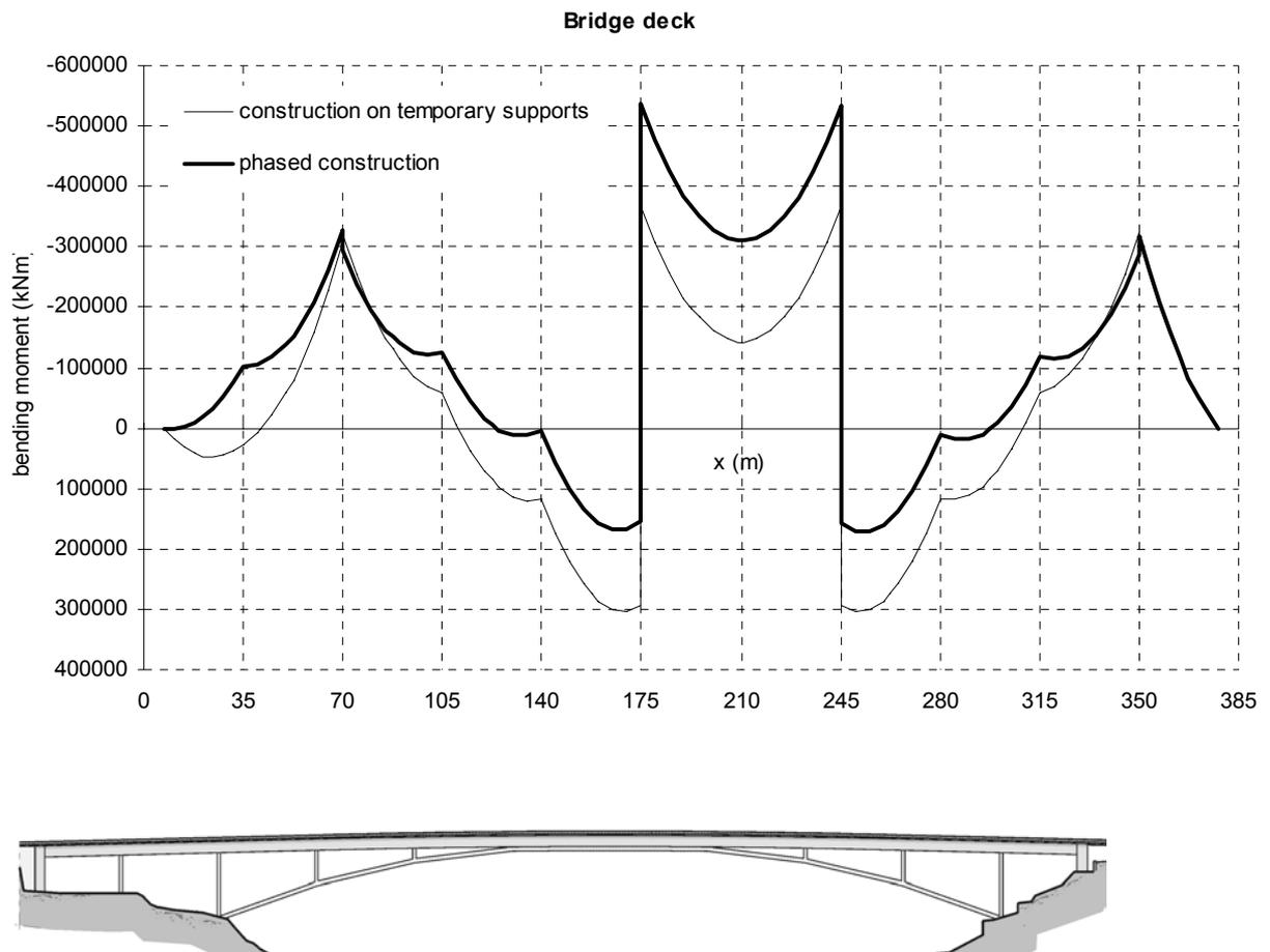
Figure 6 – Comparison of the bending moment diagrams
