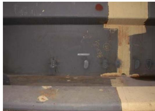
**Fig. 4.7: Inductive displacement transducers on the box-girder webs**
