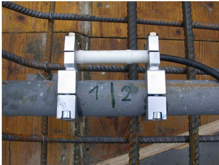
**Fig. 4.4: Strain gauge on one of the rods of the metal tie of valley bridge Albrechtsgraben**
