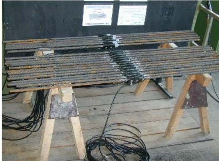
**Fig. 4.6: Reinforcement bars with especially protected strain gauges**
