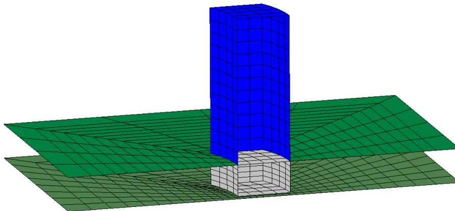
Figure 11. Example of the meshes used for the analysis. Due to symmetry, only half problem needs to be meshed.
