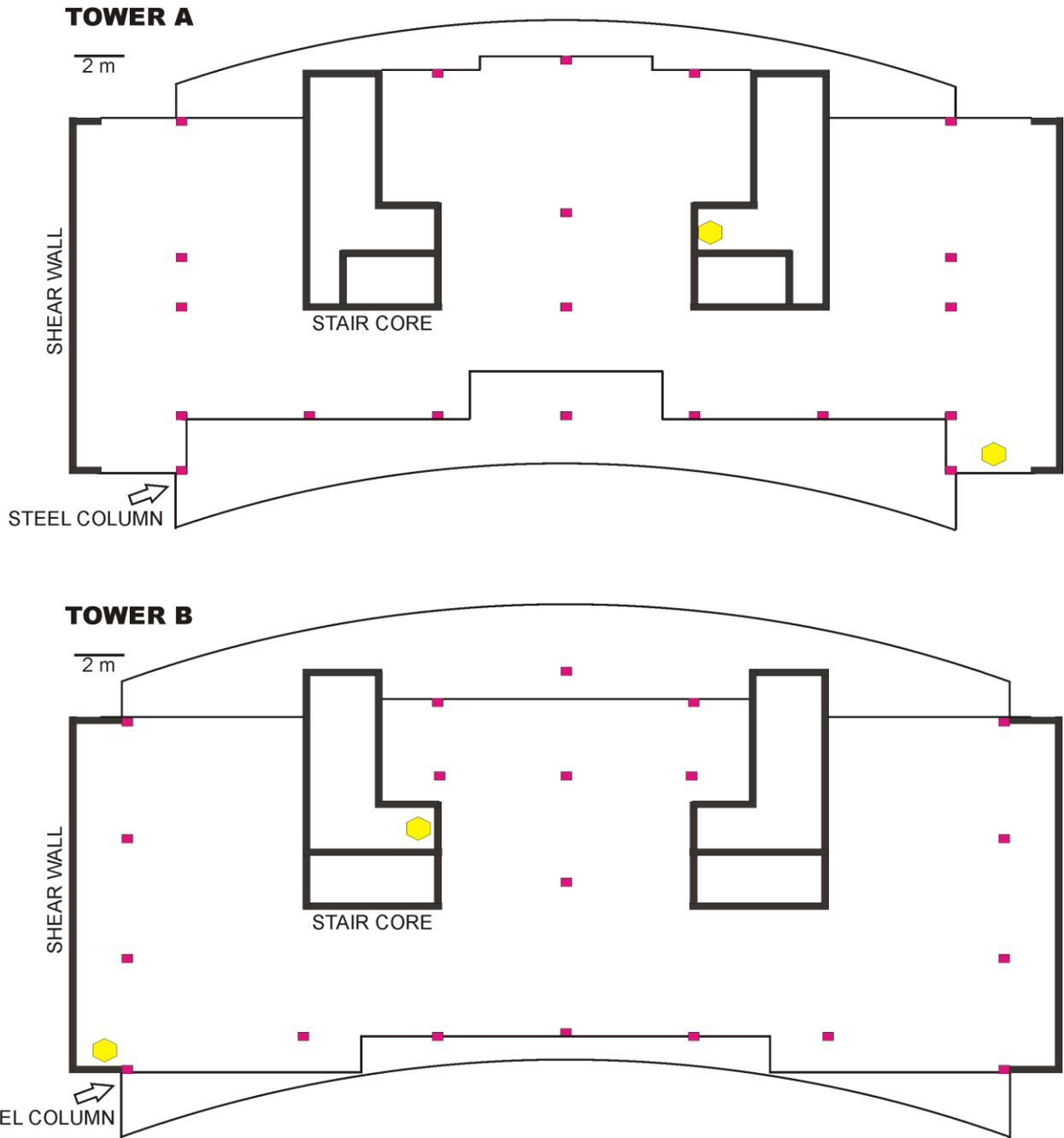
Figure 3. Structural elements of the two towers. Shear walls (thick lines) and steel double-T columns (magenta rectangles). The yellow hexagons indicate the vertical alignment of instruments inside the towers. On each even level two recordings were taken: one approximately in a barycentric position (compatible with the accessibility of the tower at the different levels) and one in a peripheral position.
