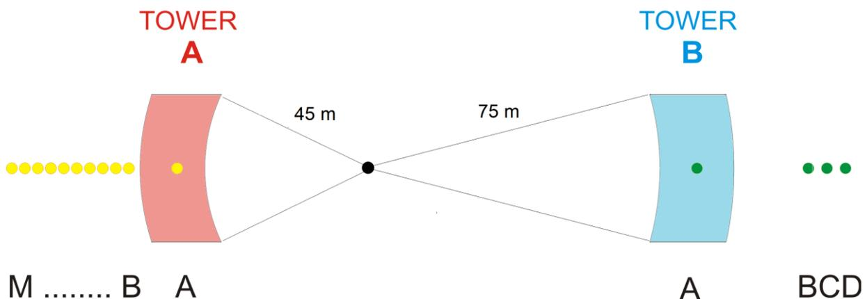
Figure 2. Schematic drawing of the tower plants that highlights their slightly different curvature ray, hardly perceptible to the sight, which is however mostly an architectural rather than a structural feature. The dots (A, B, C... M) indicate the alignment of the measurements on the ground for tower A (yellow) and B (green). See also
