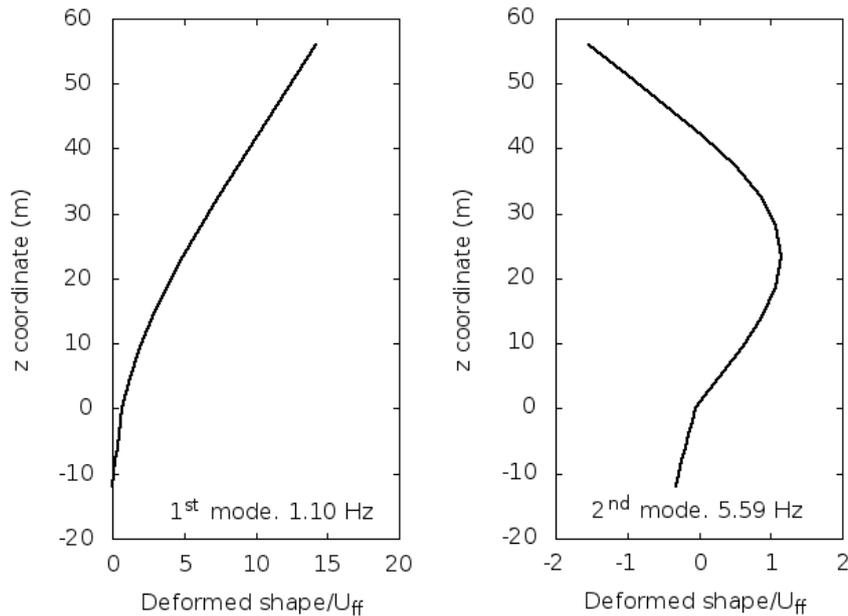
Figure 12. First and second flexion mode for tower A according to the numerical model.
