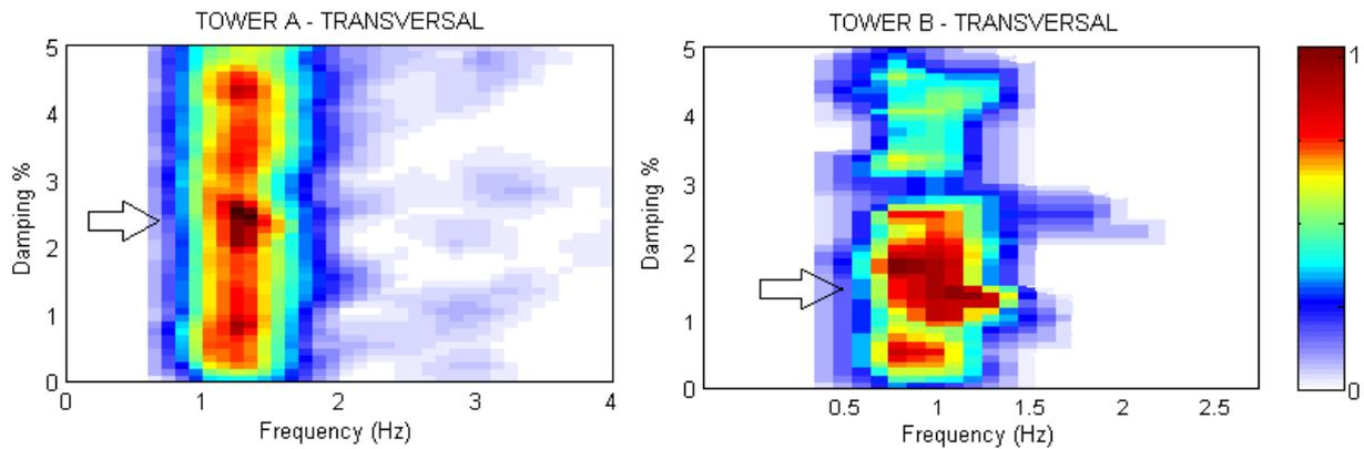
Figure 8. Damping estimated for the first flexural mode in the transversal direction for tower A (left) and B (right).
