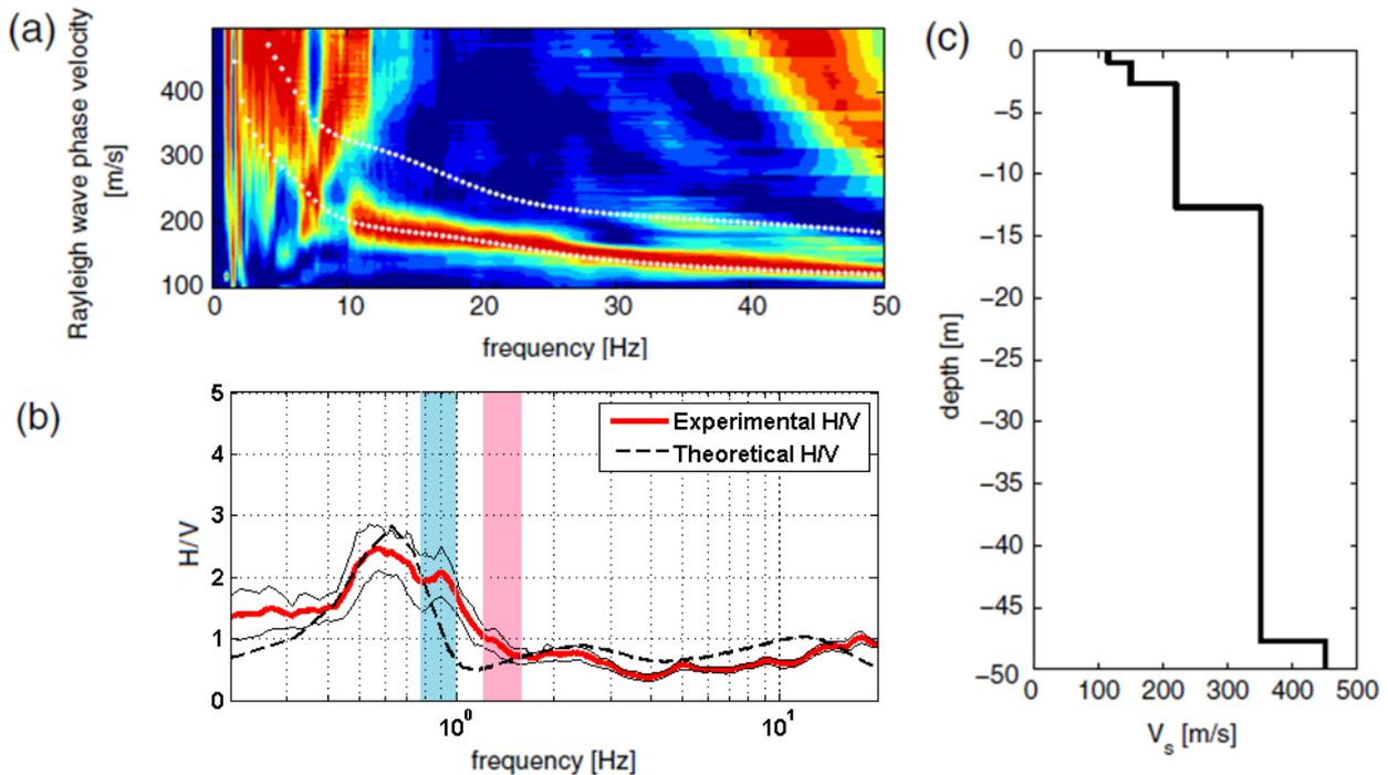
Figure 9. A) Rayleigh phase velocity spectra recorded on the free-field surrounding the towers, B) average H/V curve (red)  $\pm$  standard deviation (thin black line) of the site. The shaded areas represent the frequency of the first flexion mode of tower A (red) and B (light blue).
