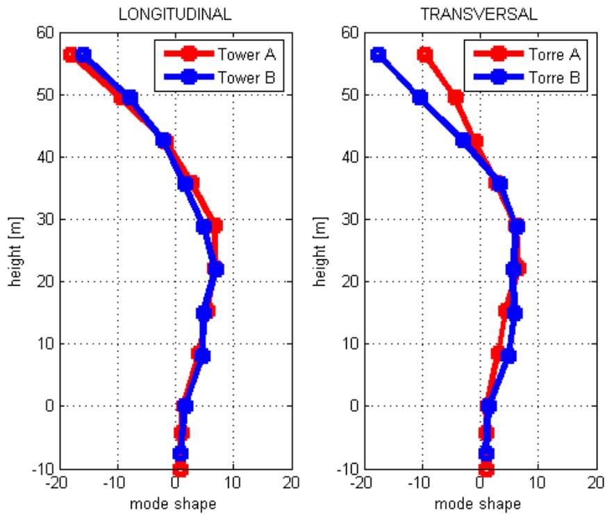
Figure 7. Second flexion mode shapes (normalized to the foundation level) of tower A and B in the longitudinal and transversal direction.
