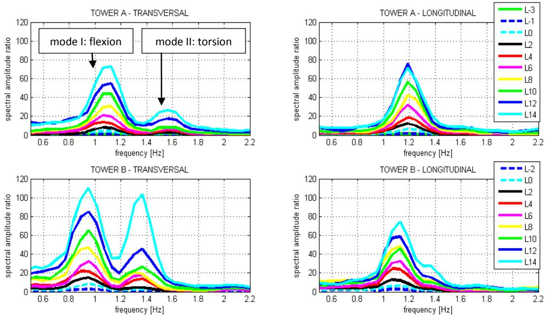
Figure 5. Modal frequencies of towers A and B obtained from the ratio of the spectra recorded at the different levels and those at the reference level (foundation floor). We observe that the behavior along the longitudinal axis is rather similar, while a substantial difference (both in terms of frequency and amplitude) appears on the transversal axis.
