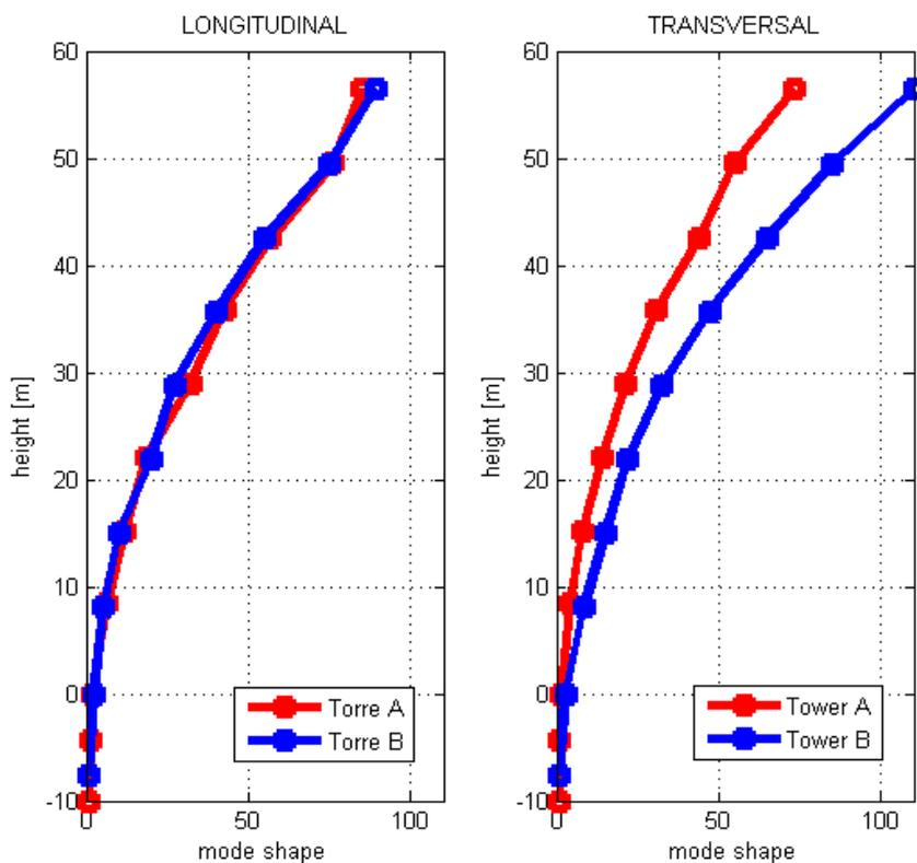
Figure 6. First flexion mode shapes (normalized to the foundation level) of tower A and B in the longitudinal and transversal direction.
