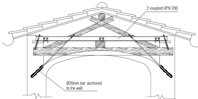
Figure 5 – Graffette method for the consolidation of a barrel vault.
