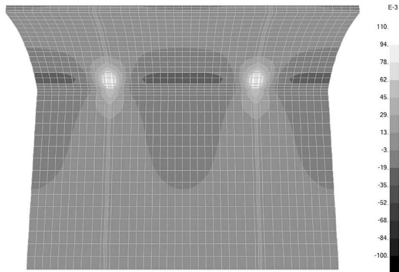
Figure 14 – Longitudinal stresses  $\sigma_y$  [N/mm<sup>2</sup>] at the intrados of the vault/wall (consolidated case with  $s=6m$ ,  $d=5m$ ,  $t=0.4m$ ).
