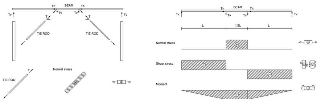
Figure 6 – Distribution of stresses in the clamp system elements.
