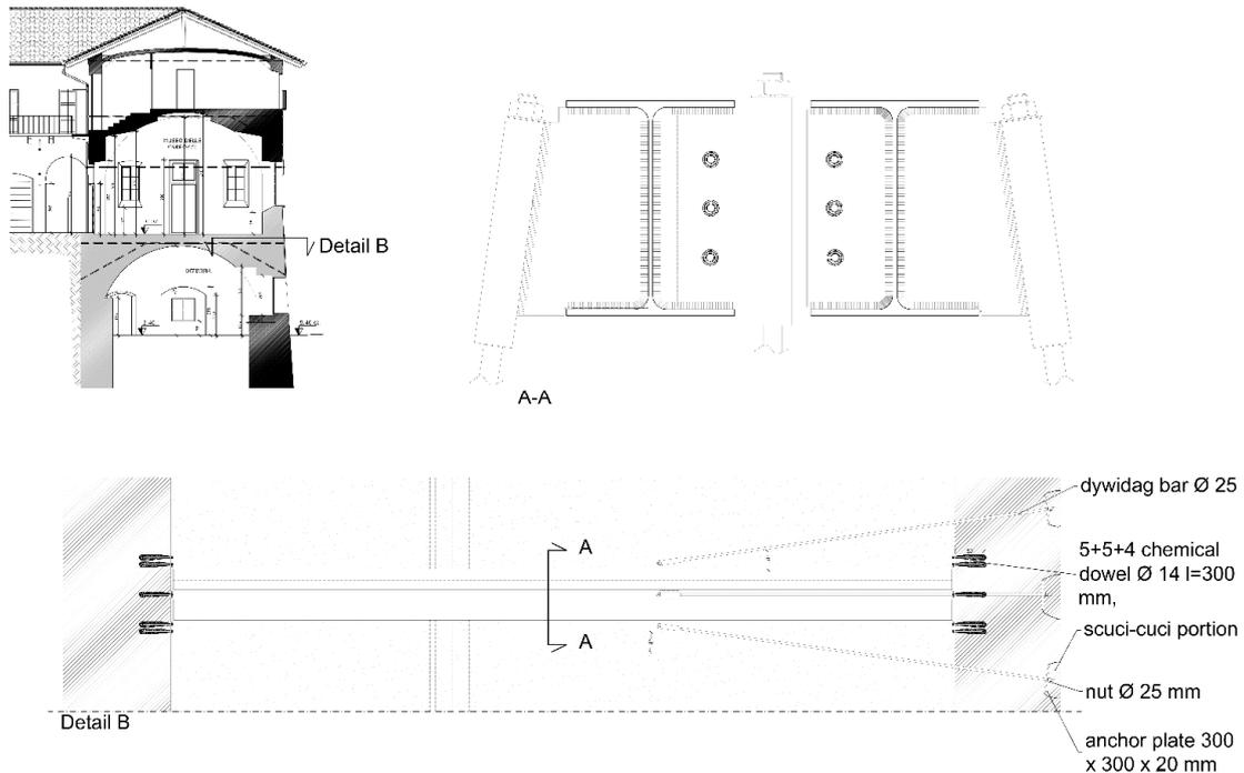
Figure 7 – Details of the consolidation with the new clamp technique on the vault of Palazzo delle Carrozze in Masino Castle, Caravino (Italy).
