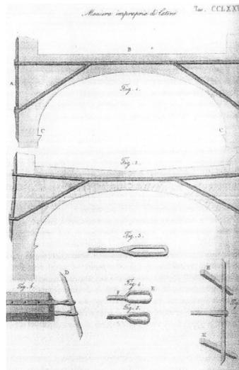
Figure 2 – Drawings from Dotti's manuscript on the braga chain, showing the elevated deformability of the horizontal element.
