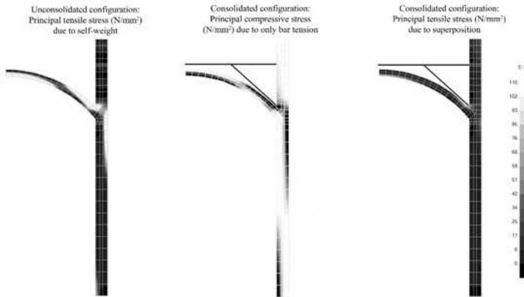
Figure 13 – Results on half transversal section of the vault, with the application of 72.5 kN on the diagonal bars.
