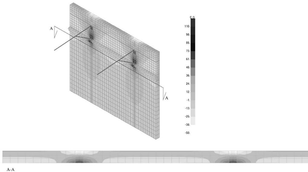
Figure 15 – Longitudinal stresses  $\sigma_y$  [N/mm<sup>2</sup>] showing a relieving arch formed between clamps (consolidated case with  $s=6\text{m}$ ,  $d=5\text{m}$ ,  $t=0.4\text{m}$ , horizontal section at the impost of the vault).
