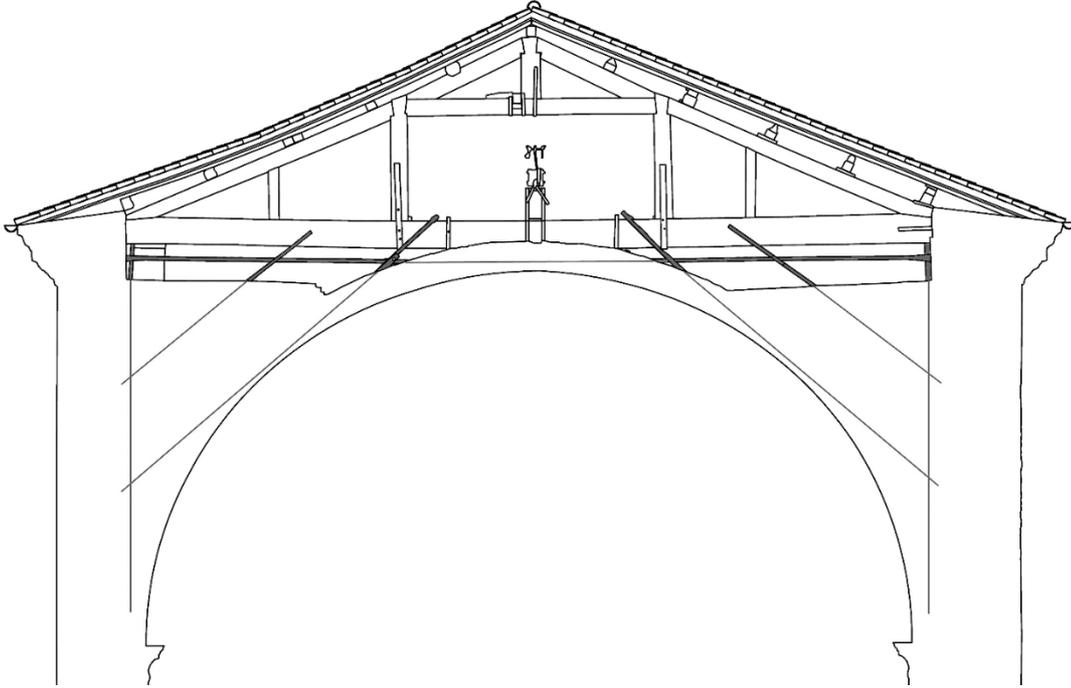
Figure 4 – Consolidation with the braga chain of the vaulted roof of San Nicolò church in Verona.
