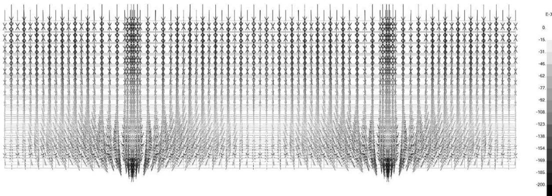
Figure 16 – Principal compressive stress arrows [N/mm<sup>2</sup>] seen from the top of the vault. Notice the concentration in correspondence with the clamps (consolidated case with  $s=6\text{m}$ ,  $d=5\text{m}$ ,  $t=0.4\text{m}$ , section at the impost of the vault).
