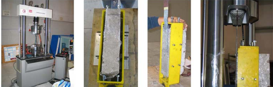
Fig. 27: Testing of the bonding force in the universal machine by direct shear
