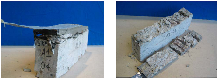
Fig. 29: Debonding by deep original concrete shear crushing failure
