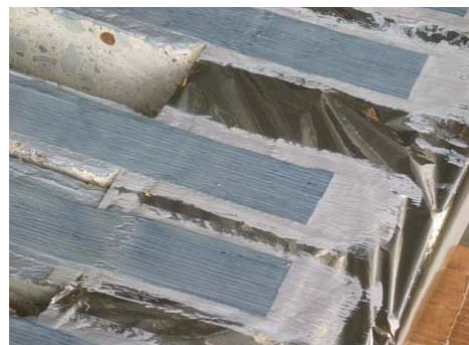
Fig. 25: Restoration of the specimen surface and application of the FRP
