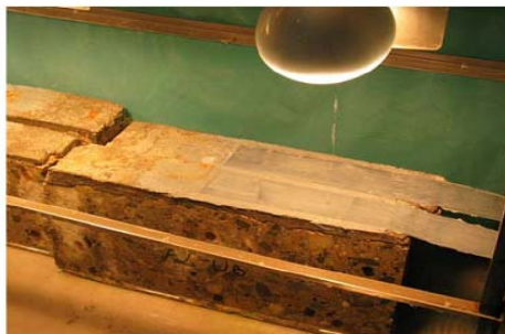
Fig. 26: Accelerated ageing of the specimen by UV rays and water moisture
