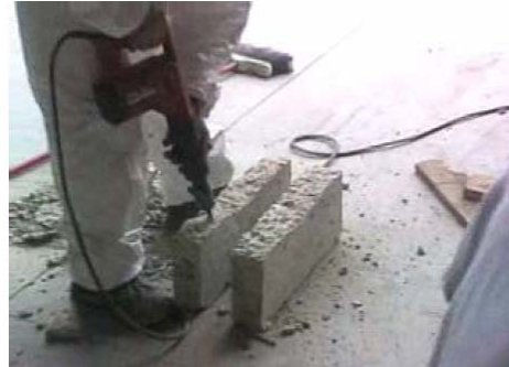
Fig. 24: Preparation of the slab specimens
