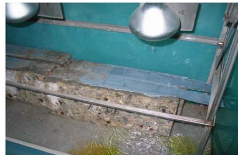
Fig. 26: Accelerated ageing of the specimen by UV rays and water moisture
