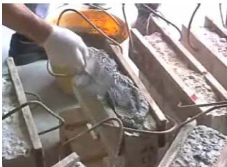
Fig. 25: Restoration of the specimen surface and application of the FRP
