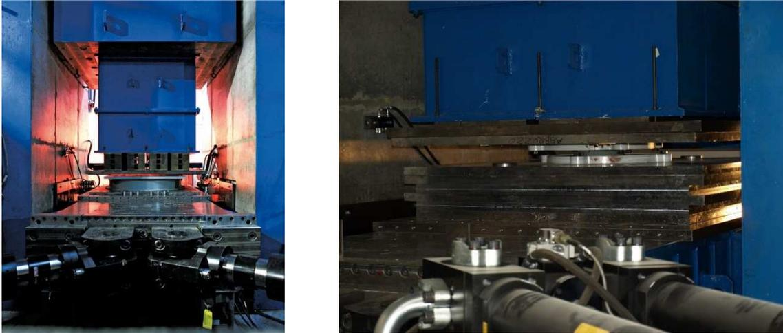
Figure 5: TREES Lab of Eucentre Bi-axial Bearing Tester Machine (left) and a DCCSS under test in it (right).
