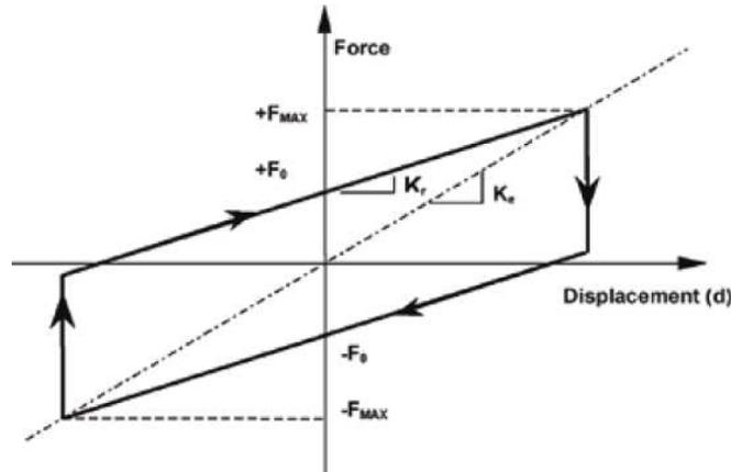
Figure 2: Theoretical force vs. displacement graph of CSS or DCCSS.
