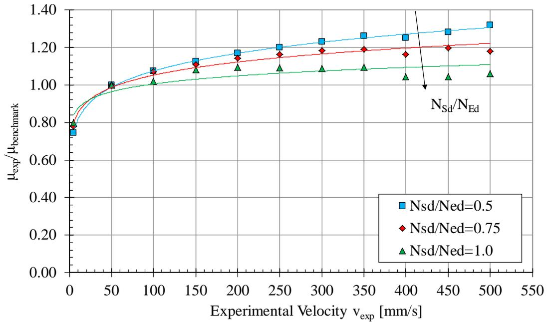
Figure 12: Normalized dynamic friction coefficient vs. test velocity
