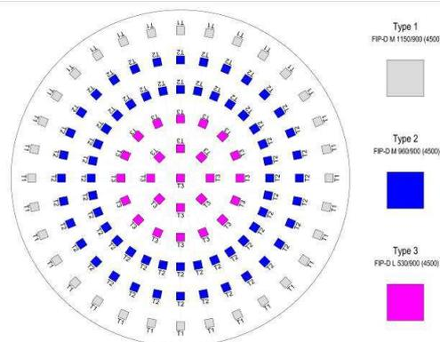
Figure 19: Ammonia storage tank in Samsun, Turkey: seismic isolators layout plan.
