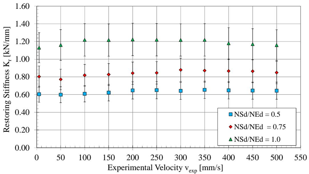
Figure 13: Restoring stiffness vs. test velocity
