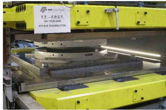
Figure 3: FIP Biaxial Dynamic Test Facility (left) and a DCCSS under test in it (right).
