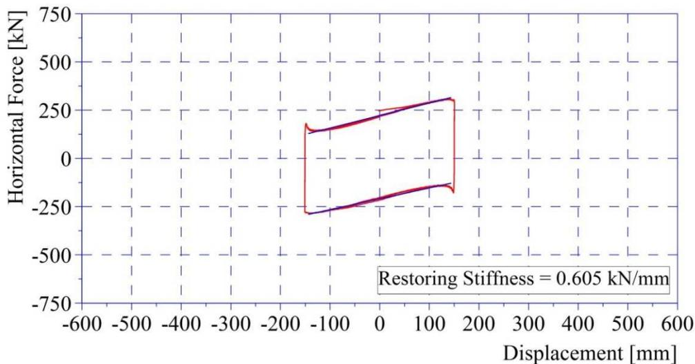
Figure 11: Benchmark Test – experimental force vs. displacement graph on double concave curved surface slider FIP-D M 1450/470(3100).
