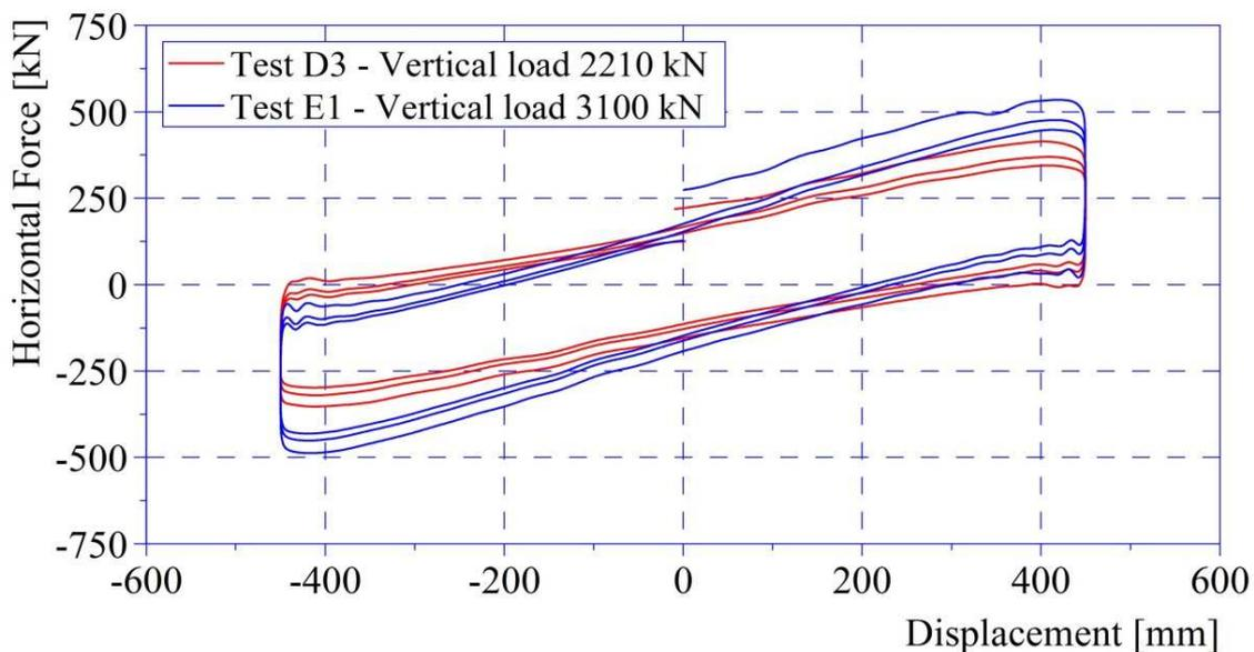
Figure 8: Experimental Force vs. displacement graph of the double concave curved surface slider FIP-D M 1150/900(4500) tested at two different loading conditions
