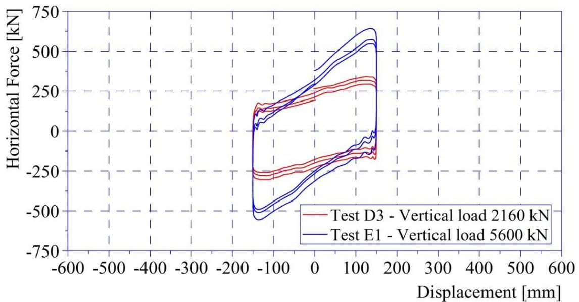
Figure 9: Experimental Force vs. displacement graph of a double concave curved surface slider FIP-D M 1450/470(3100) tested at two different loading conditions.
