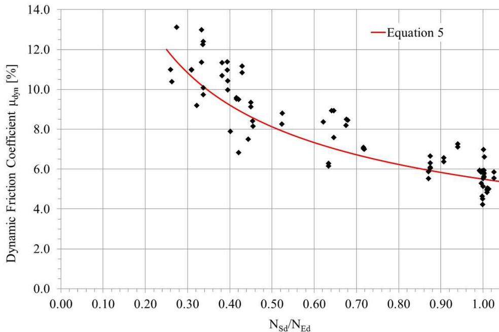
Figure 7: Experimental dynamic friction coefficient variation with the vertical load.
