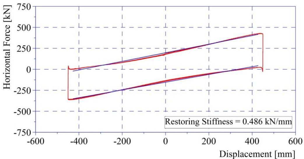
Figure 10: Benchmark Test – experimental force vs. displacement graph on double concave curved surface slider FIP-D M 1150/900(4500)
