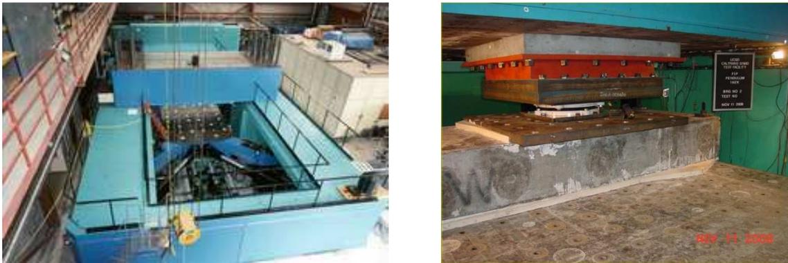
Figure 6: Caltrans SRMD Test Facility (left) and a DCCSS under test in this machine (right).
