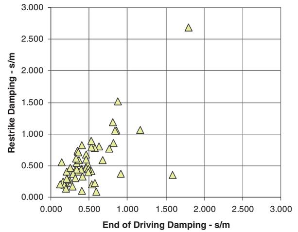
Figure 4. Combined damping factor J-comb (BOR vs EOD) for the 55 selected cases.
