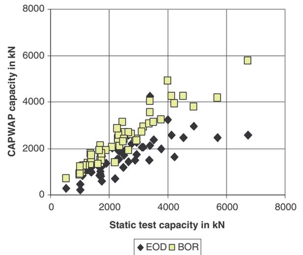
Figure 2. Correlation of CAPWAP capacity with static load test capacity for 55 cases selected for the damping and quake study.
