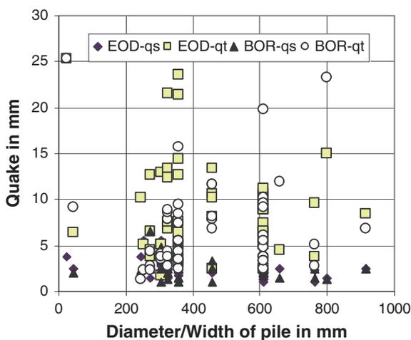
Figure 5. CAPWAP calculated toe quakes vs pile diameter or width for the 55 selected cases.
