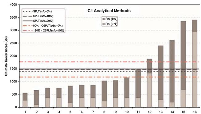
Figure 1. Comparison of capacities from analysis of driven pile and static load test on companion pile – after Viana da Fonseca and Santos (2003).
