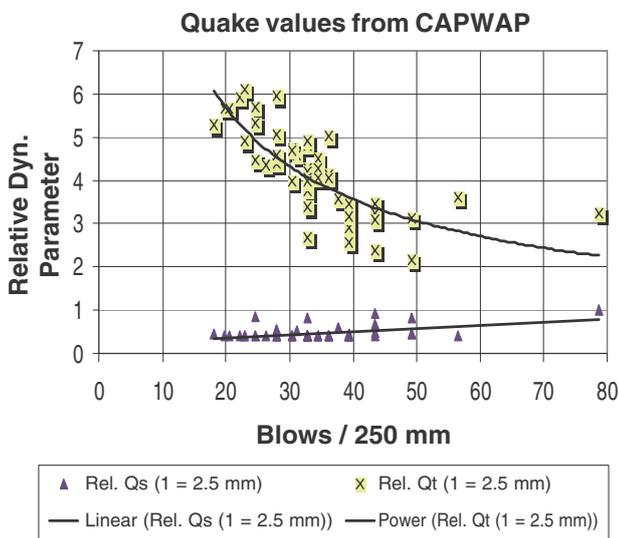
Figure 9. Quake values for 42 piles at the same site.
