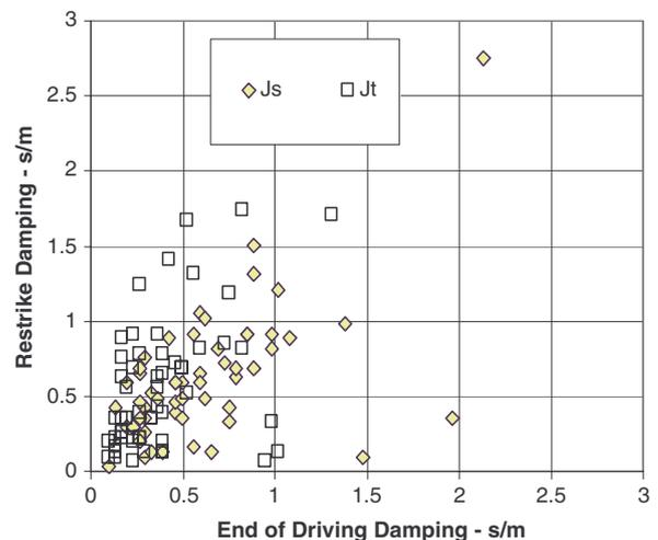
Figure 3. Shaft and toe damping factors: EOD vs BOR from 55 tests.
