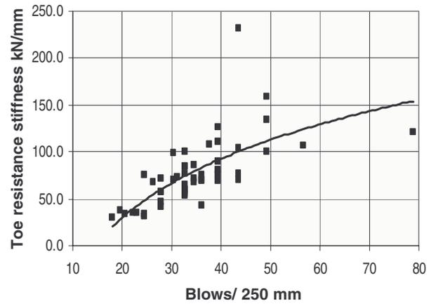
Figure 10. Toe resistance stiffness in shale for 42 piles at the same site.
