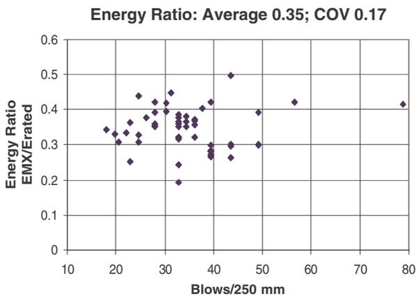
Figure 7. Energy transfer ratio vs blow count for 42 piles at the same site.
