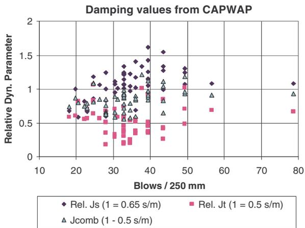
Figure 8. Damping values for 42 piles at the same site.
