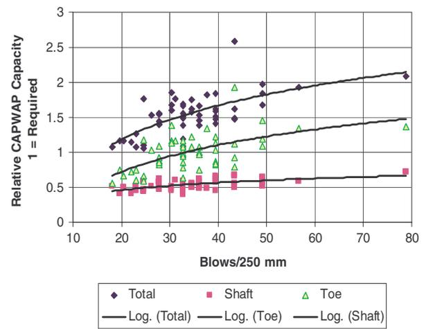
Figure 6. CAPWAP capacity results for 42 piles at the same site.
