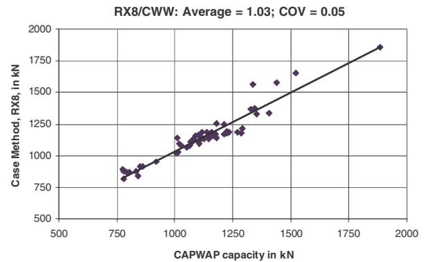
Figure 14. Simplified vs Signal Matching for 42 cases at the same site.
