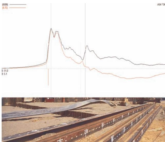
Figure 11. Example of a twisted H-pile (below) and the associated EOD record of force (upper curve) and velocity vs time.
