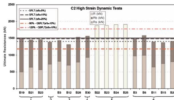
Figure 13. Comparison of capacities from signal matching of dynamically tested pile and static load test on companion pile after Viana da Fonseca and Santos (2003).
