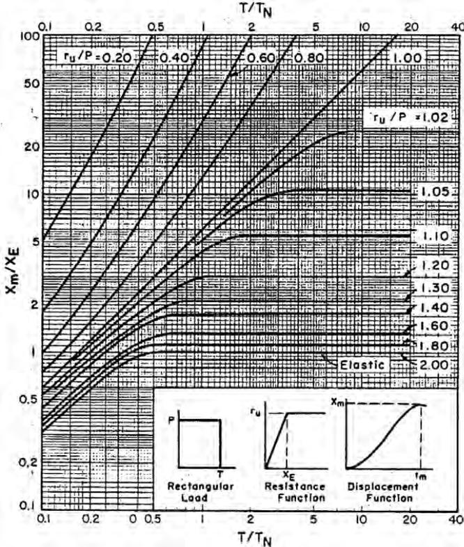
Fig. 7: Chart to calculate maximum deflection response  $X_m$  (from [10] fig. 3.56) attained at time  $t_m$ . The blast load is defined by its duration  $T$  and peak value  $P$ . The SDOF elastic deflection is  $X_E$  and  $r_u$  is its ultimate resistance, finally its natural period is  $T_N$ .
