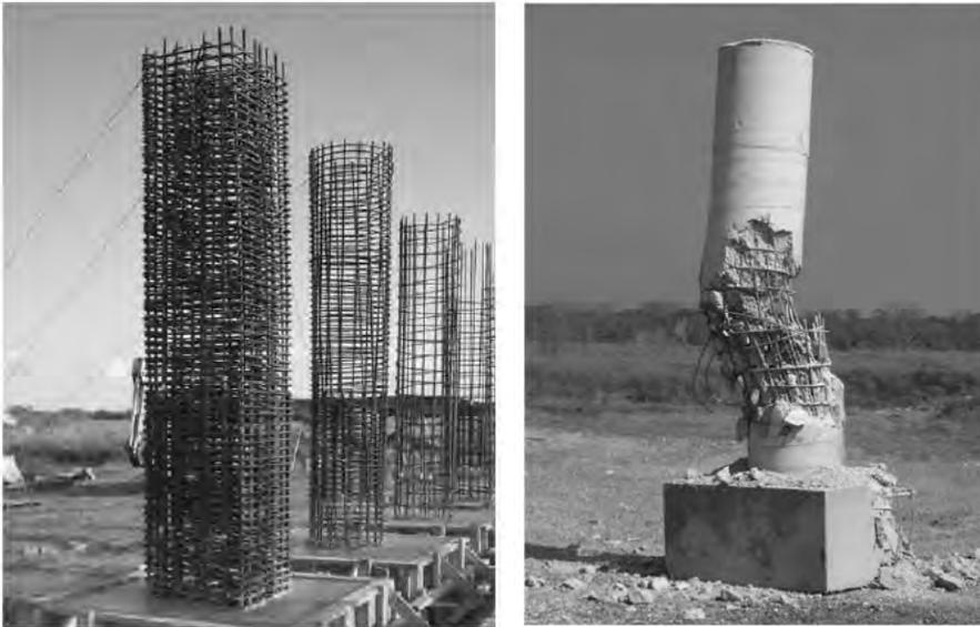
Fig. 23. Different steel cages and plastic hinge after blast.
