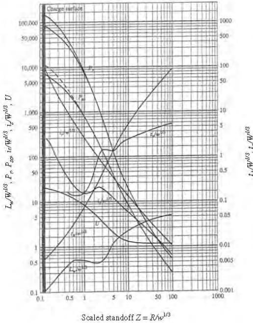
Fig. 4. Positive phase airblast parameters for hemispherical surface TNT detonation at sea level (Department of the Army, 1990).
