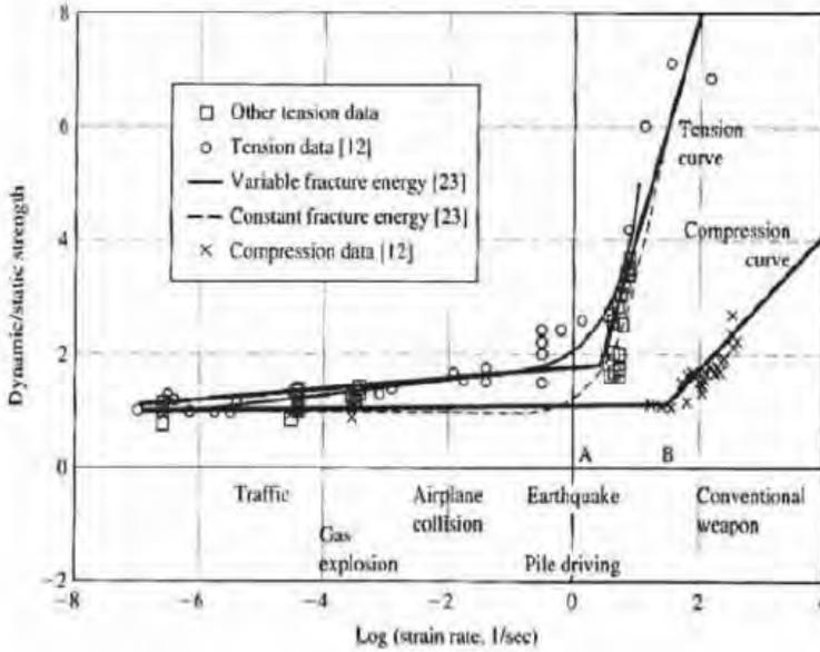
Fig. 13: Concrete strain-rate effects on strength (Tedesco 1999).
