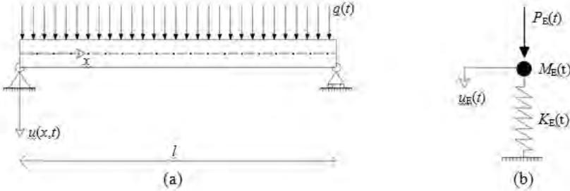
Fig. 9: (a) Real beam; (b) equivalent SDOF model of the real beam.
