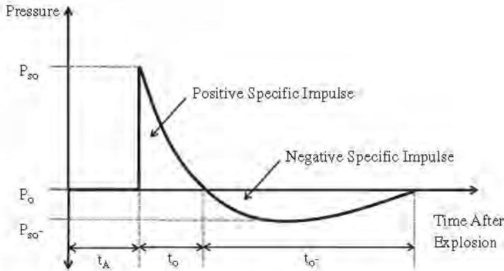
Fig. 3 Idealized pressure–time curve for free-air explosion (Department of the Army, 1990).
