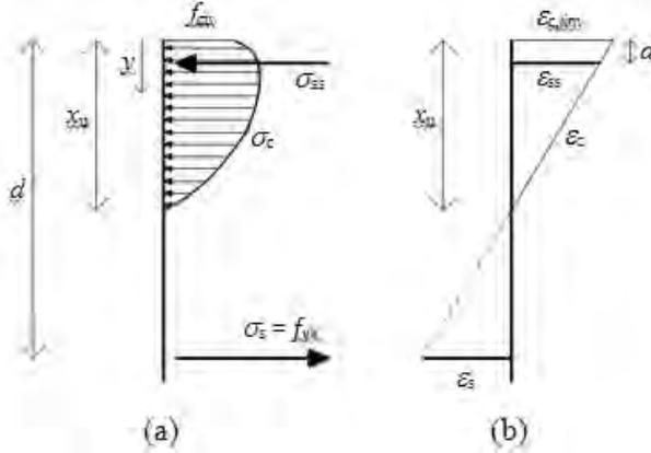
Fig. 12: (a) Stress distribution over the cross-section at the ultimate state; (b) strain diagram at the ultimate state.
