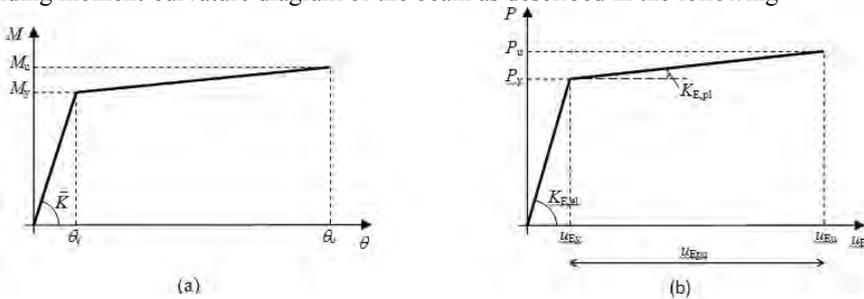
Fig. 10: (a) Bilinear bending moment-curvature diagram of the beam; (b) corresponding bilinear load-displacement diagram of the equivalent SDOF model.
