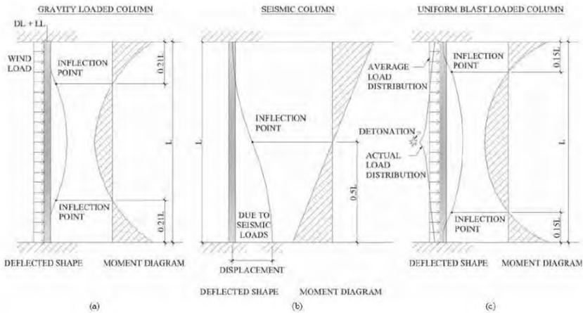
Fig. 19. Moment diagram and detected shape for each load case: a) typical, b) seismic, c) blast.
