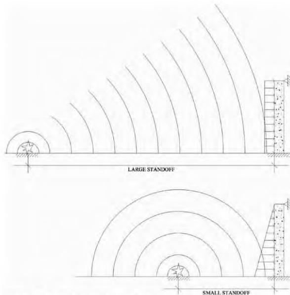
Fig. 20. Blast load distribution versus standoff.
