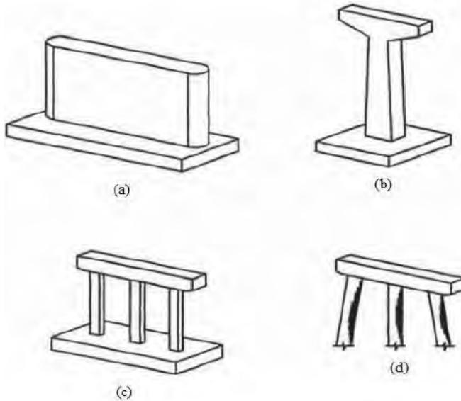
Fig. 18. Typical column types: a) solid, b) single column, c) multi-column, d) pile bent (NYSDOT, 2006).
