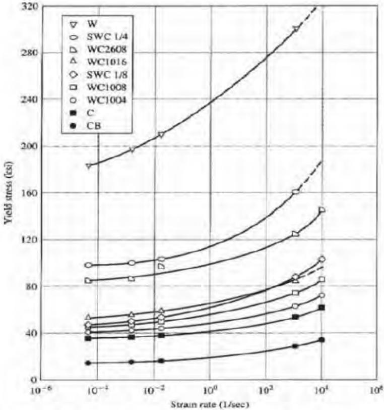
Fig. 14: Effects of strain-rate on yield stress for various metals (Tedesco 1999).
