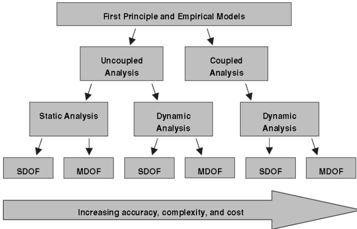
Fig. 17. Flowchart of possible analysis methods (Winget, 2003).
