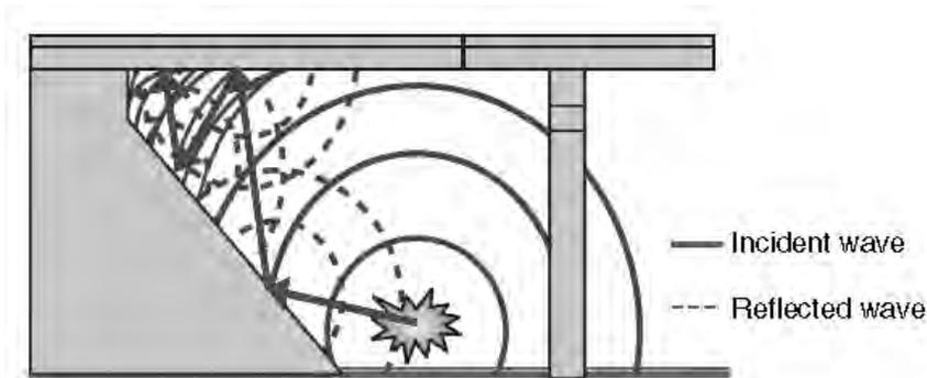
Fig. 6. Blast-wave propagation during below-deck explosion (Winget et al., 2005).
