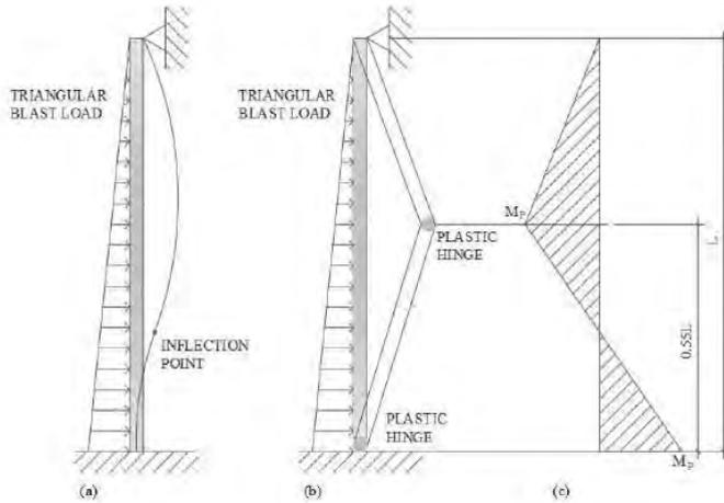
Fig. 21. Plastic hinge analysis for blast-loaded column: a) detected shape, b) plastic hinge locations, c) plastic moment.
