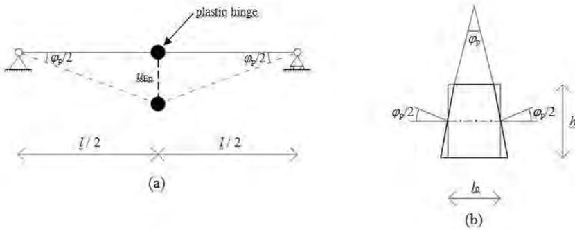
Fig. 11: (a) Plastic deflections of the beam with a concentrated plastic hinge at the mid-span section; (b) schematic representation of the plastic hinge.
