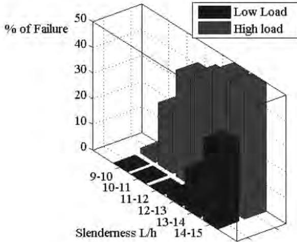
Fig. 16. Collapse percentage of the beams examined with reference to both load scenarios.
