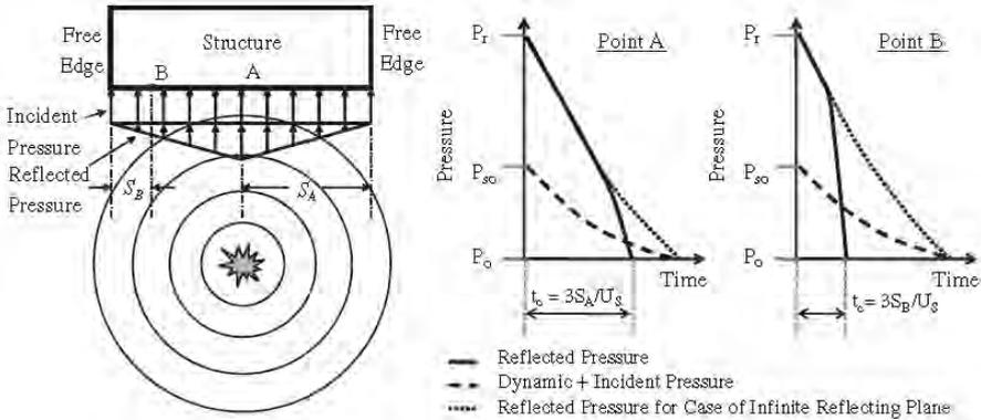
Fig. 5. Blast wave reflecting off structure (U.S. Army Engineer Research and Development Center, 2003).
