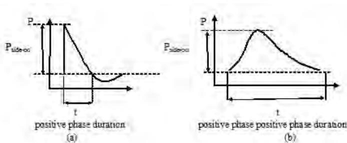
Fig. 2: Pressure time-histories for detonation (a) and deflagration (b).
