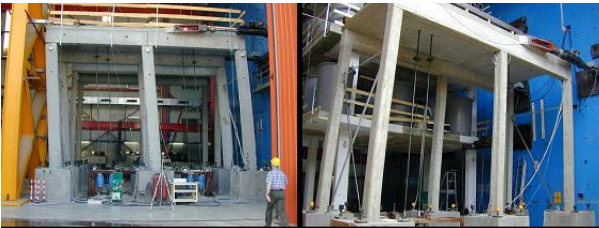
Fig. 2. Precast and cast-in-situ prototypes during the tests.
