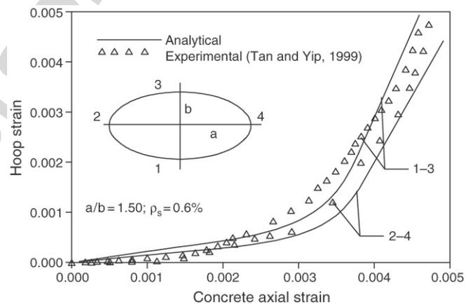
Fig. 9. Experimental and analytical variation in hoop strain with concrete axial strain.
