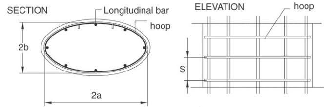
Fig. 1. Typical details of column.
