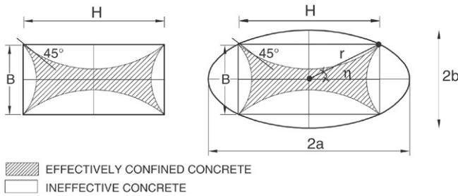
Fig. 7. Effective confined area in rectangular and elliptical transverse cross-sections.
