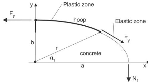
Fig. 6. Equilibrium condition of a portion of the confined section.
