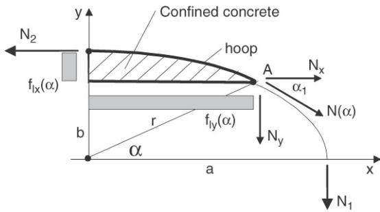
Fig. 3. Equilibrium condition of a portion of the confined cross-section.
