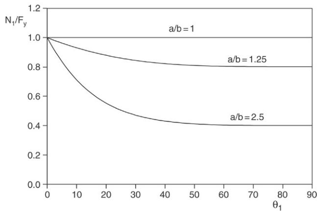
Fig. 10. Analytical dimensionless variation of axial force  $N_1$  with the plasticization angle  $\theta_1$ .
