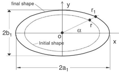
Fig. 5. Lateral expansion of confined cross-section.
