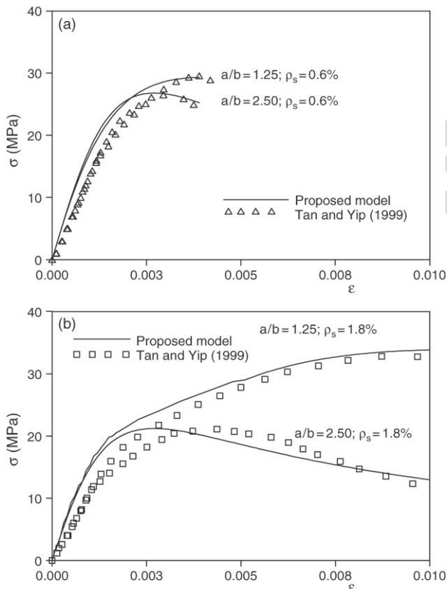
Fig. 8. Comparison between analytical and experimental stress–strain curves. (a) Low volumetric ratio ( $\rho_s = 0.6\%$ ); (b) high volumetric ratio ( $\rho_s = 1.8\%$ ).
