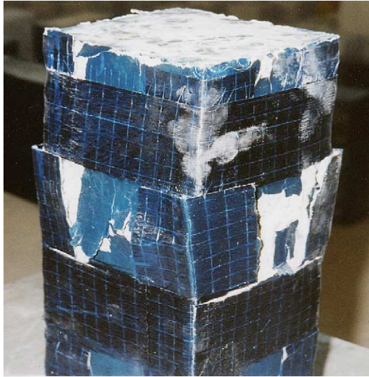
Fig. 4. Failure mode of CFRP discontinuously wrapped specimens.
