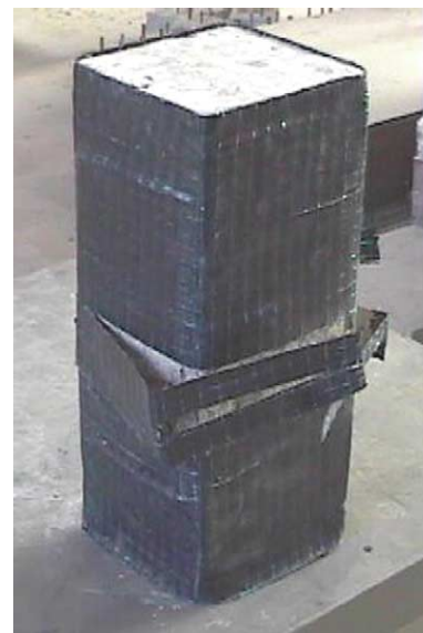
Fig. 3. Failure mode of CFRP continuously wrapped specimens.
