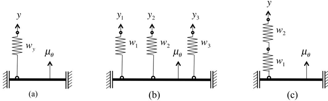
**Fig. 1.** Mechanical analogy of simple linear Gaussian inference problems: parameter estimation based on one observation (a), three uncorrelated observations (b), one observation affected by three uncorrelated sources of uncertainty (c).
