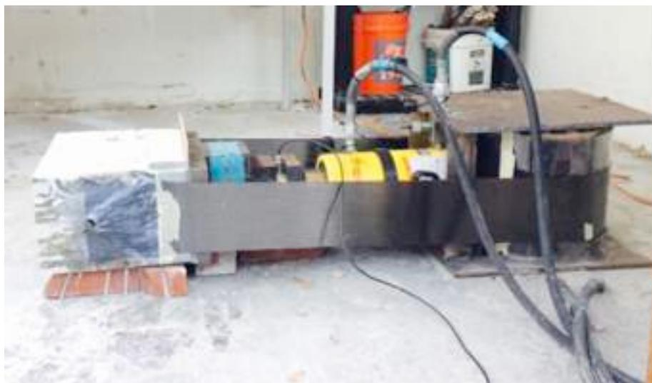
**Figure 9 - Test 3 – Double Shear Test**
